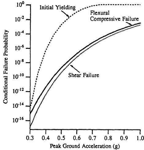
Figure 3 Seismic fragility function
