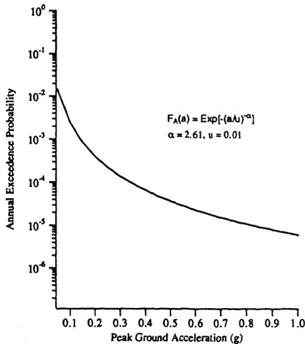
Figure 4 Seismic hazard function
