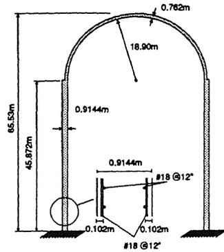
Figure 1 Reinforced concrete containment structure
