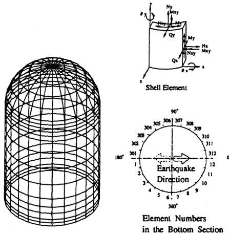
Figure 2 Finite element model
