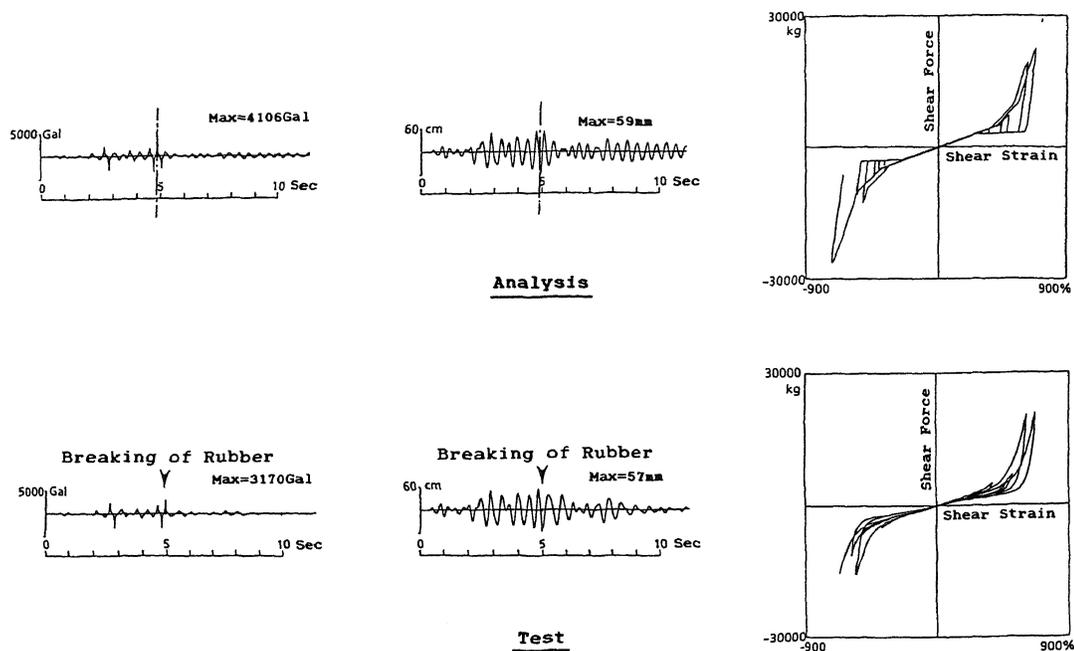
Fig.9 Simulation Analysis Result
