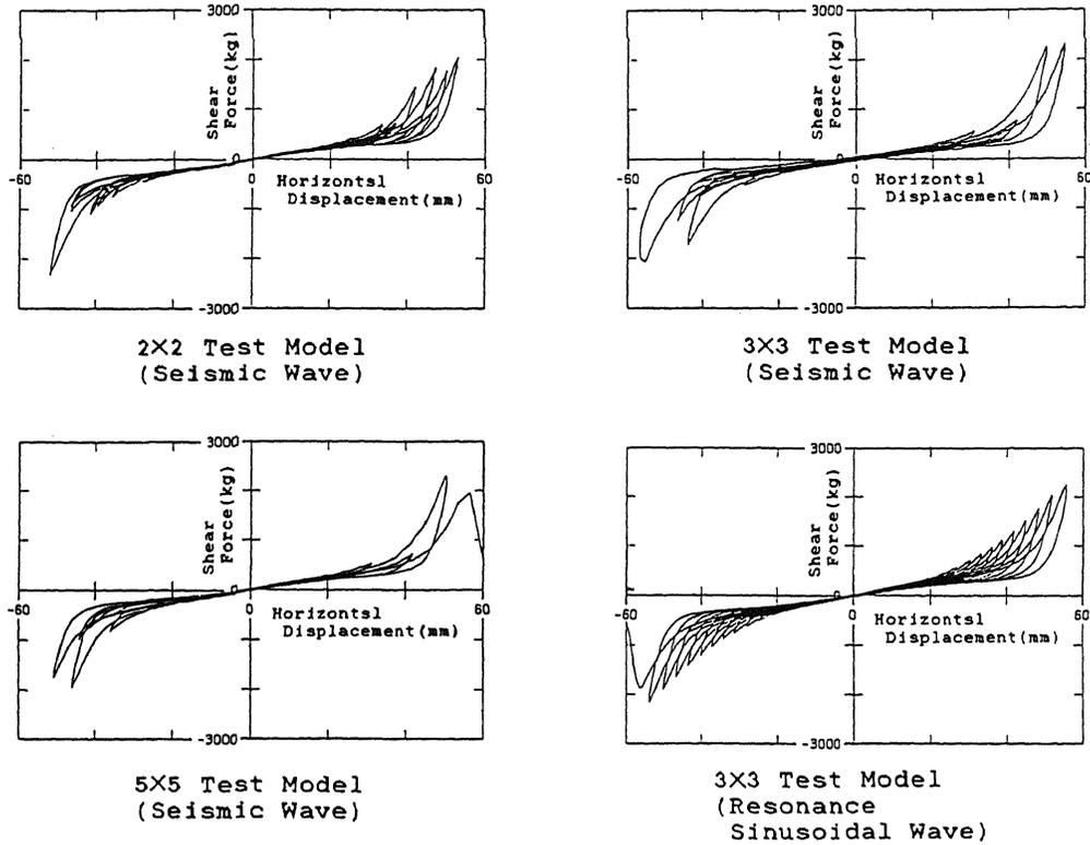
Fig.5a Shear Force-Horizontal Displacement of SIL
