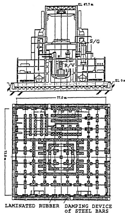
Fig.1 Seismic Base Isolated Reactor Building for FBR Plant
