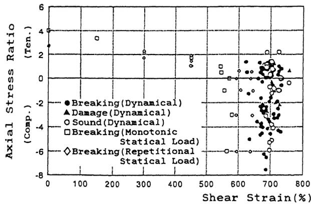
Fig.5b Maximum Stress-Strain Relation of Laminated Rubber Specimen
