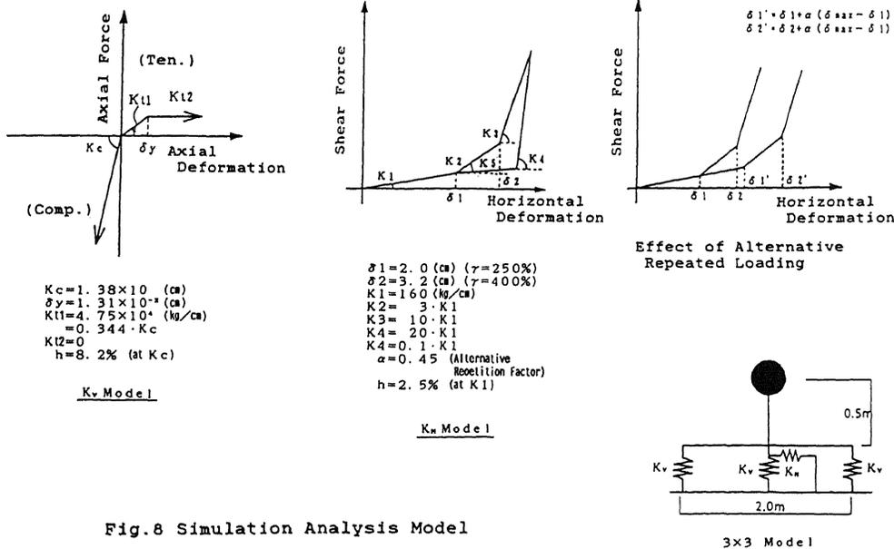
Fig.8 Simulation Analysis Model
