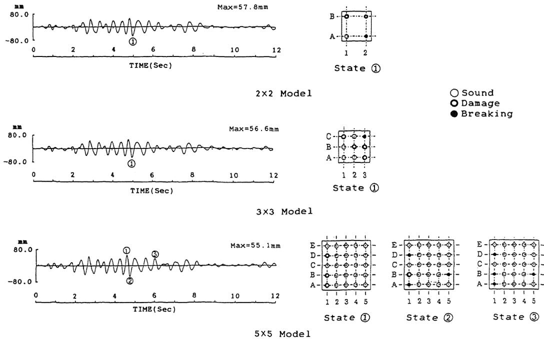
Fig.6 Breaking Mode of Laminated Rubber Specimen
