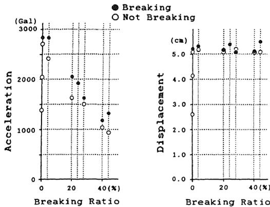
Fig.7 Breaking Ratio-Response of SIL
