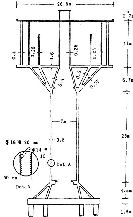
Figure 4. Dimensions of tank 2
