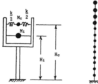
Figure 7. TDOF model Figure 8. Beam model
