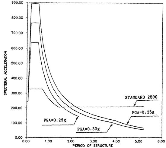
Figure 5. Spectral accelerations
