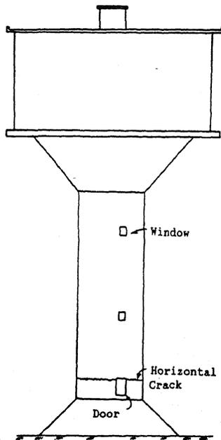
Figure 3. Elevation of tank 2
