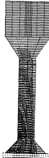
Figure 11. Flexural stress distribution
