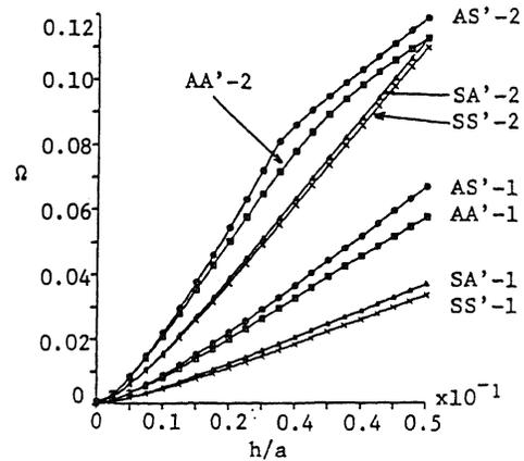
Figure 5. Variation of natural frequency  $\Omega$  with thickness-to-radius ratio ( $h/a$ ).
