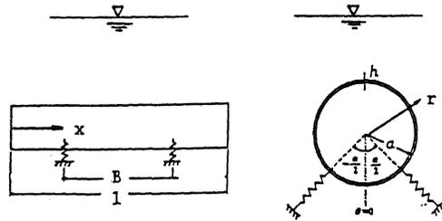
Figure 1. Elastically point-supported cylindrical shell in fluid medium.
