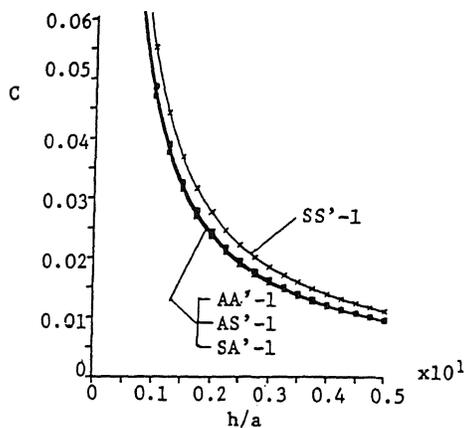
Figure 8. Variation of added mass factor  $C$  with thickness-to-radius ratio ( $h/a$ ).
