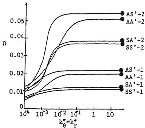
Figure 3. Variation of natural frequency  $\Omega$  with stiffness  $k_{\theta}^* = k_r^*$ .
