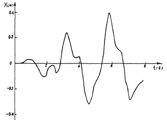
Fig. 5 Displacement response of the smokestack.
