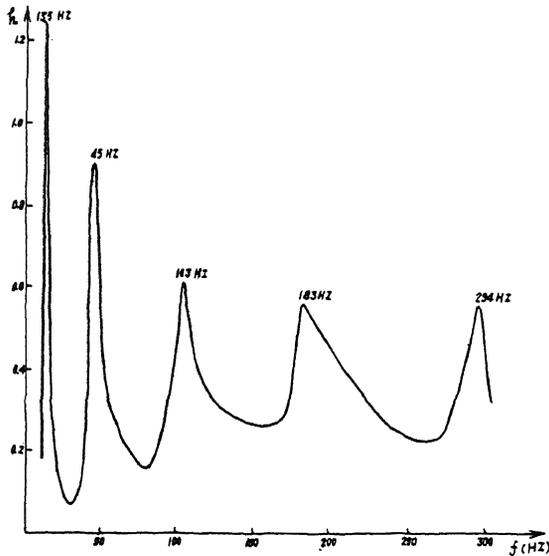
Fig. 2 Resonance curve of the model
