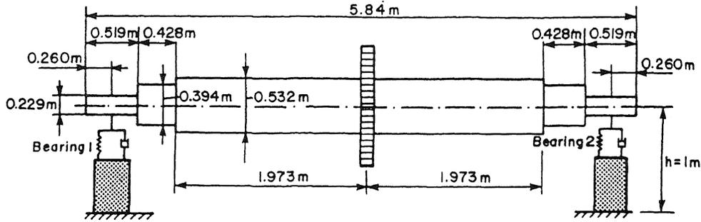
Figure 1: Rotor-Disk-Bearing System considered in the study.
