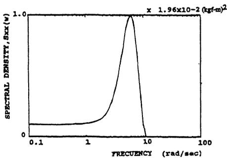
Figure 4. R/C beam response spectral density function.
