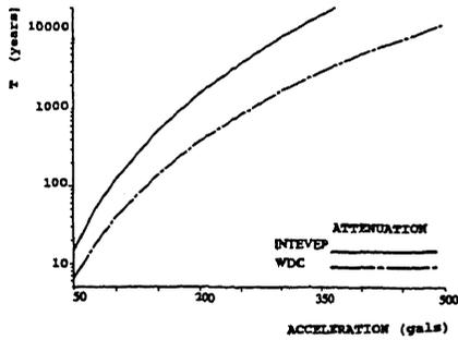
Figure 3. Peak ground acceleration vs. return period.
