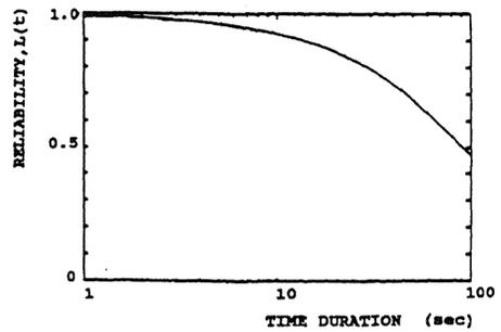
Figure 6. Platform structural reliability.
