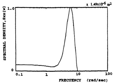
Figure 7. Equipment displacement response spectral density function.
