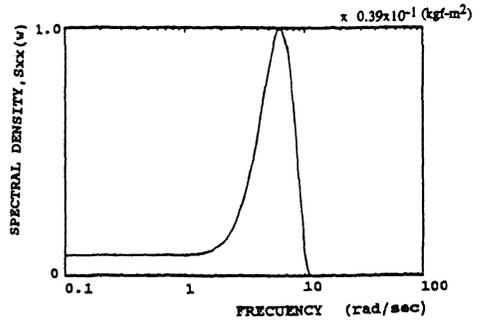
Figure 5. Pile response spectral density function.
