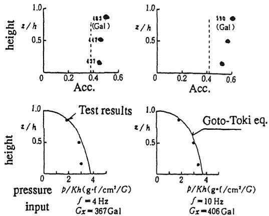
Fig. 4. Distributions of Acc. and Hydrodynamic pressures around Model
