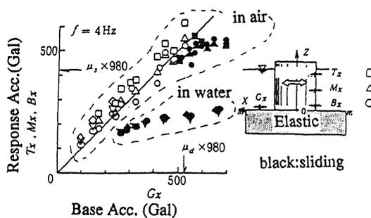
Fig. 6. Comparison of Acc. in water and in air
