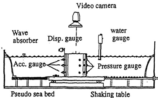
Fig. 1. Underwater Shaking table test devices
