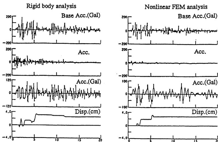
Fig.10. Comparison of Response Wave forms in Rigid body analysis and nonlinear FEM analysis
