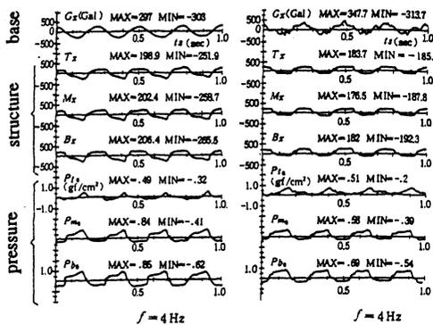
Fig. 5. Response Acc. and Hydrodynamic pressures wave forms
