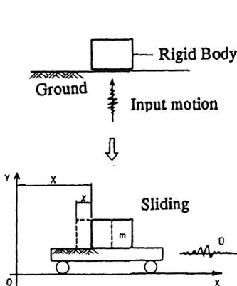
Fig. 7. Modeling of Rigid body Sliding Analysis
