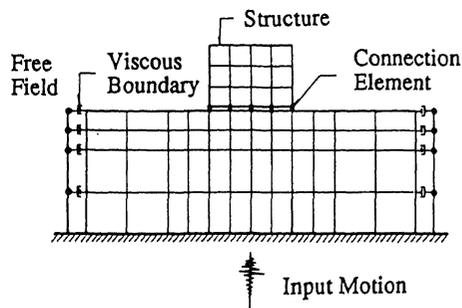
Fig. 8. Modeling of Nonlinear Dynamic FEM analysis
