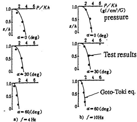
Fig. 3. Distributions of Hydrodynamic Pressures around Cylinder Model
