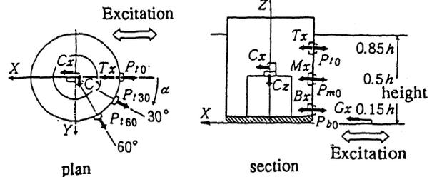
Fig.2. Measuring points of model
