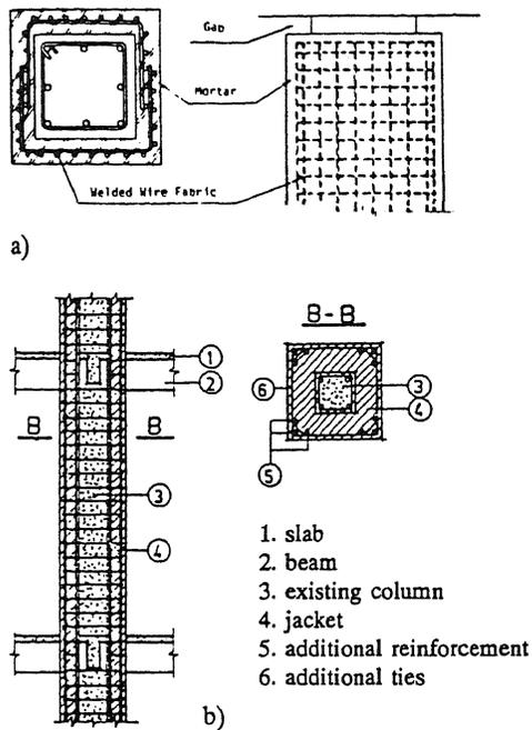
Figure 2. Types of column jacket (Sugano 1980)
