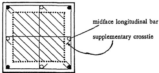
Figure 3. Midface longitudinal bars and supplementary cross ties in columns
