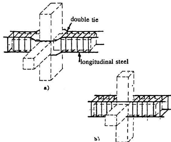
Figure 6. Continuity of longitudinal steel in jacked beams
