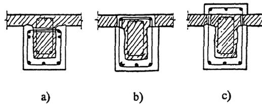
Figure 5. Three and four sides jacking of beams (Iglesias 1985)
