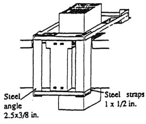
Figure 7. Structural steel cage assembled in the joint (Alcocer 1990)
