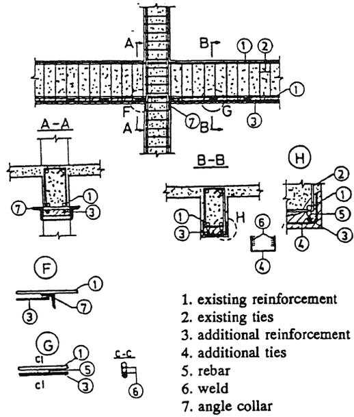
Figure 4. One side jacking of beams (UNDP/UNIDO 1983)
