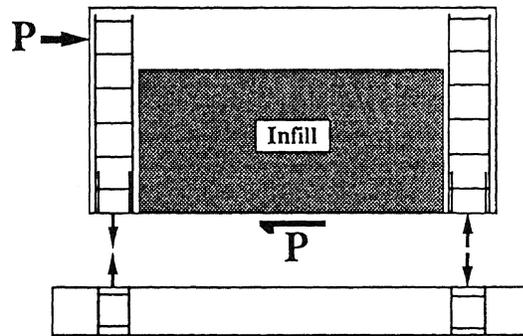
Fig. 1 Axial forces in columns resulting from overturning of infill walls
