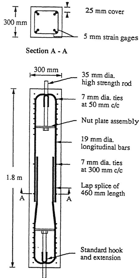
Fig. 2 Test specimen with existing (unstrengthened) splice details
