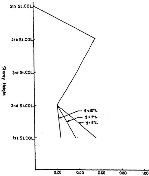
Figure 8. Zone IV column strengthening reinforcement/design reinforcement for five storey uniform building.
