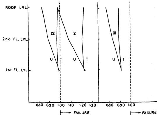
Figure 3. Ratio of checking moment to design moment for beams of three storey buildings.
