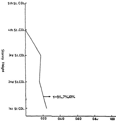
Figure 12. Zone III column strengthening reinforcement/design reinforcement for five storey tapered building.
