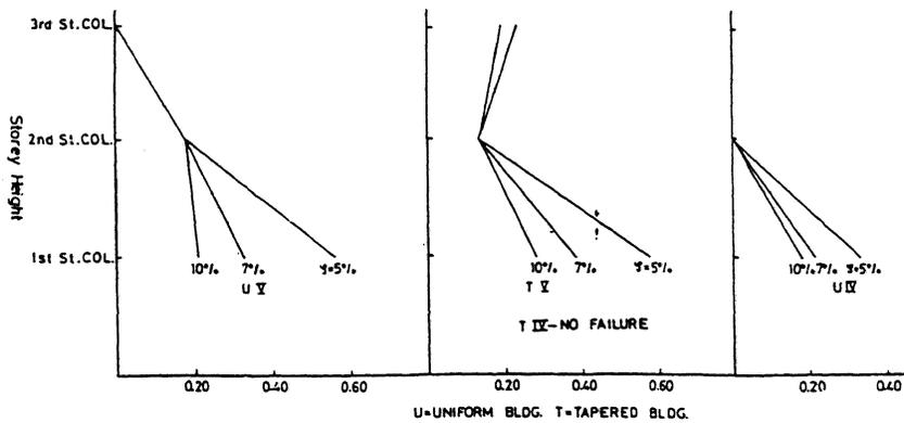
Figure 6. Column strengthening reinforcement/design reinforcement in three storey buildings.
