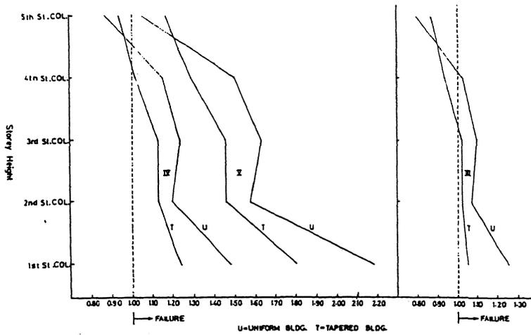
Figure 5. Ratio of checking moment to design moment for beams of five storey buildings.
