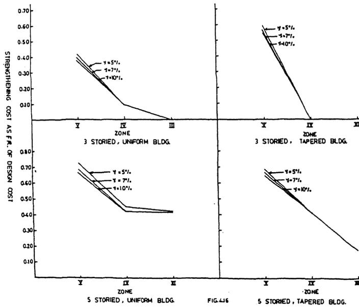
Figure 16. Strengthening cost/design cost for various buildings.
