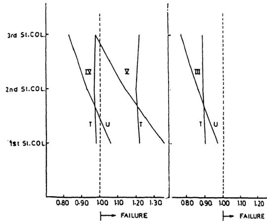
Figure 2. Ratio of checking moment to design moment for columns of three storey buildings.
