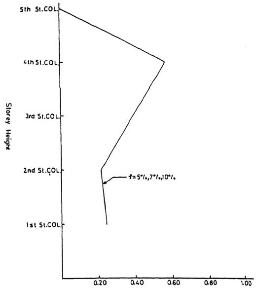
Figure 9. Zone III column strengthening reinforcement/design reinforcement for five storey uniform building.
