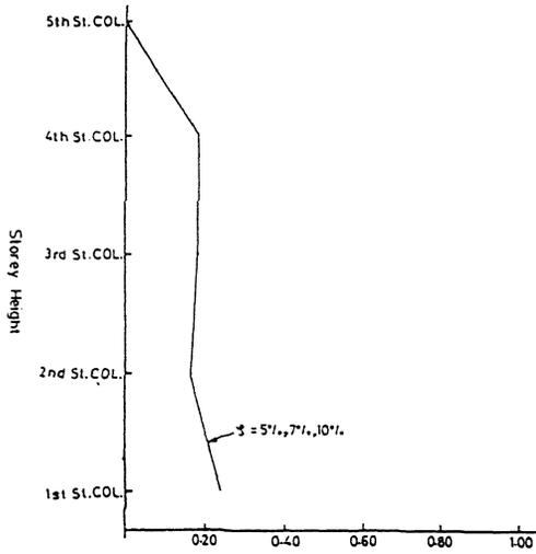
Figure 11. Zone IV column strengthening reinforcement/design reinforcement for five storey tapered building.
