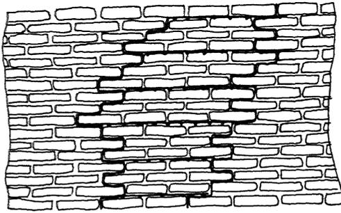
Figure 4. Masonry weaving
