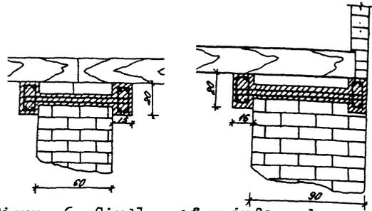
Figure 6. Girdles of reinforced concrete
