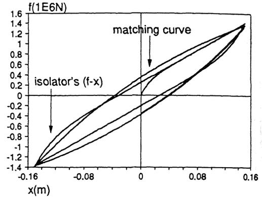
Fig. 6: force-displacement diagram of the isolator and matching curve
