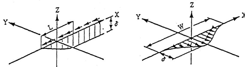
① Displacement in the direction of pipe axis
