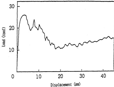
Fig.4 Load to displacement curve of threaded joint
