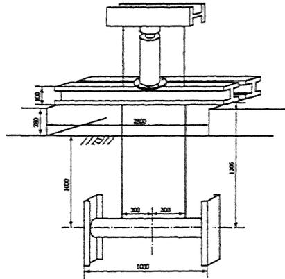
Fig.7 Measuring method of ground spring property
