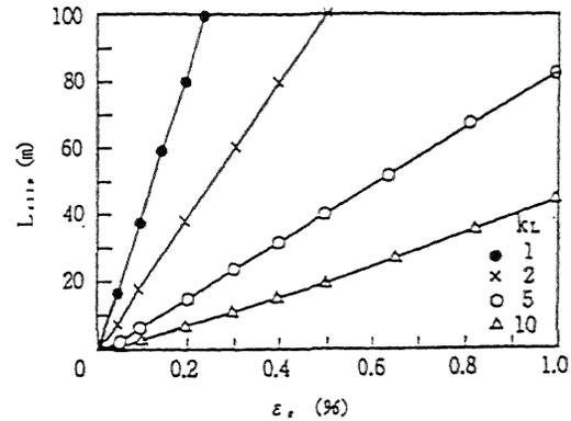
Fig.15 Slip length of semi-infinite straight conduit
