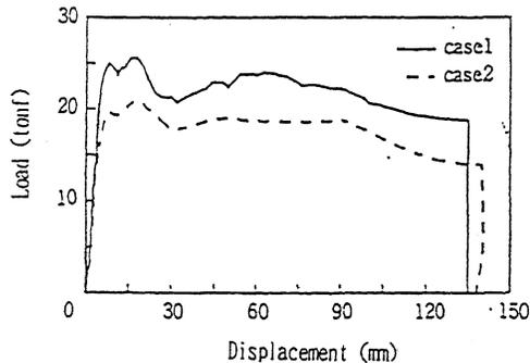
Fig.9 Load to displacement curve obtained by simulation experiment
