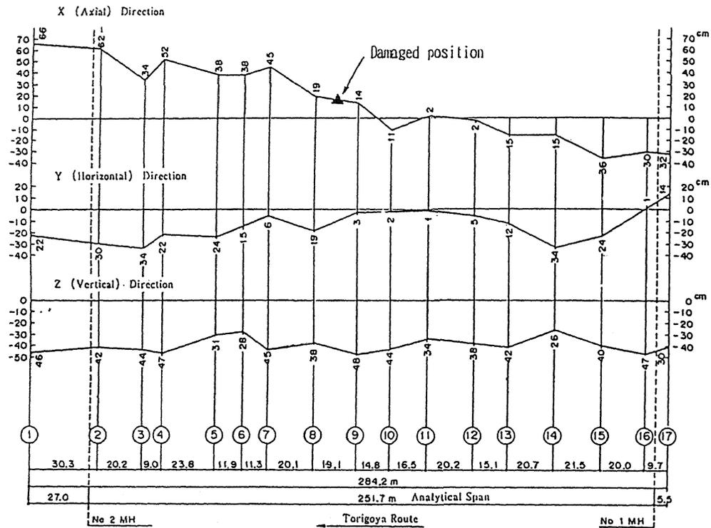
Fig.2 Distribution of permanent displacement in the damaged interval
