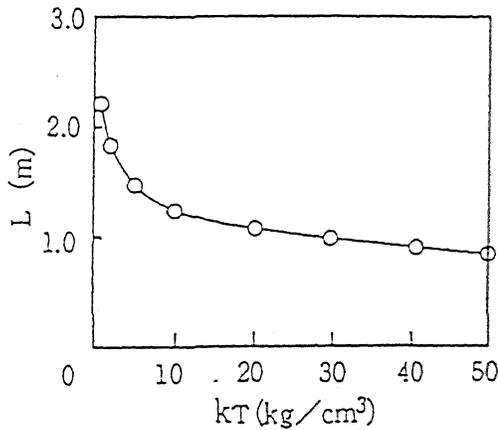
Fig.13 Buckling wave length
