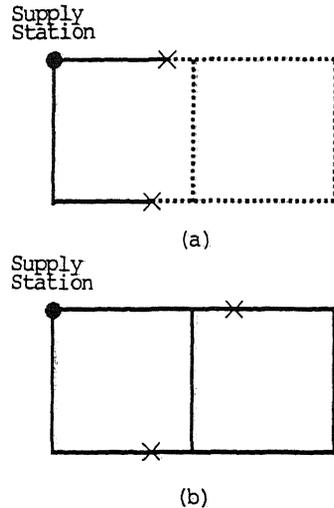
Figure 2. Definition of service ratio. (x : damaged point)
