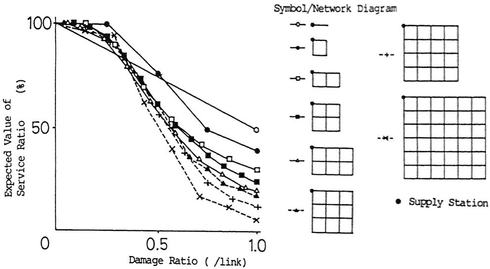
Figure 8. Damage ratio vs. service ratio for different networks.
