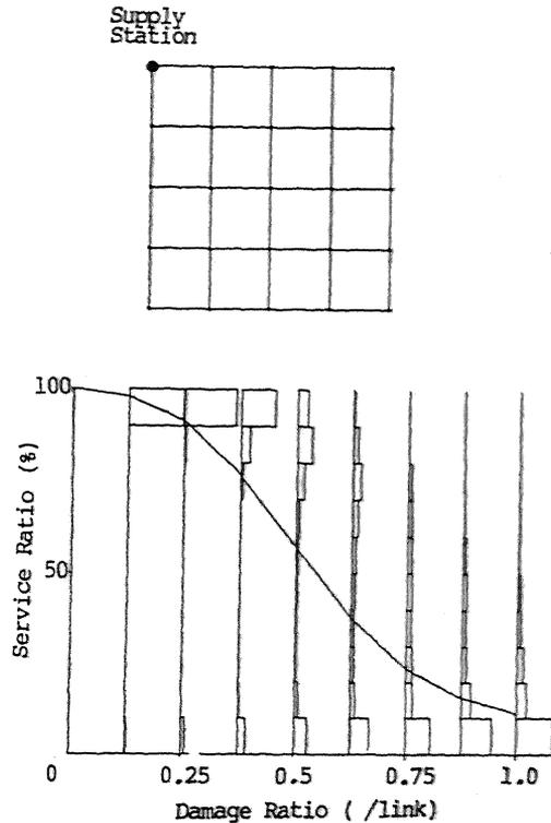
Figure 6. Damage ratio vs. service ratio for a checkerboard-type network (1000 simulations).
