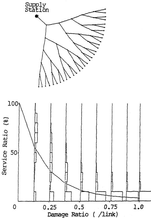
Figure 5. Damage ratio vs. service ratio for a tree-type system (1000 simulations).
