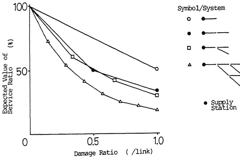
Figure 7. Damage ratio vs. service ratio for different systems.
