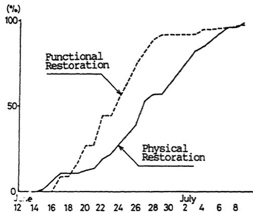
Figure 1. Restoration process of gas system in Sendai City.
