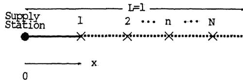
Figure 3. One-link system with a supply station at only one end.
