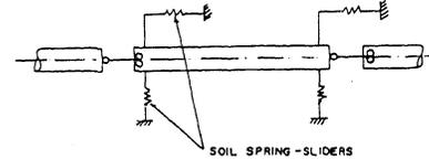
Figure 3. Pipeline model
