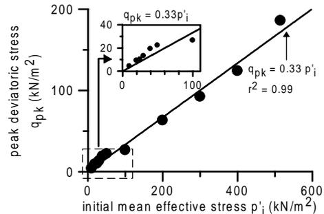
(b) Measured peak deviatoric stresses vs initial effective confining pressures
