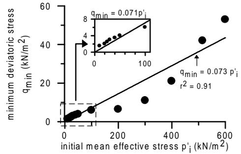
(a) Measured minimum deviatoric stresses vs initial effective confining pressures
