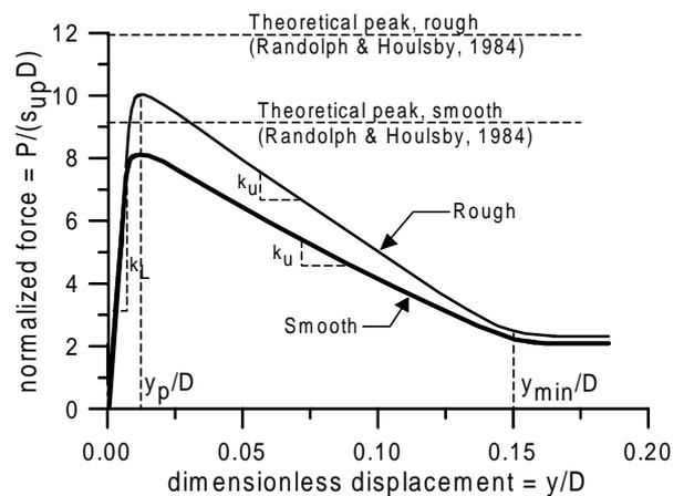
**Figure 4 Normalized Strain-Softening p-y Curve**
