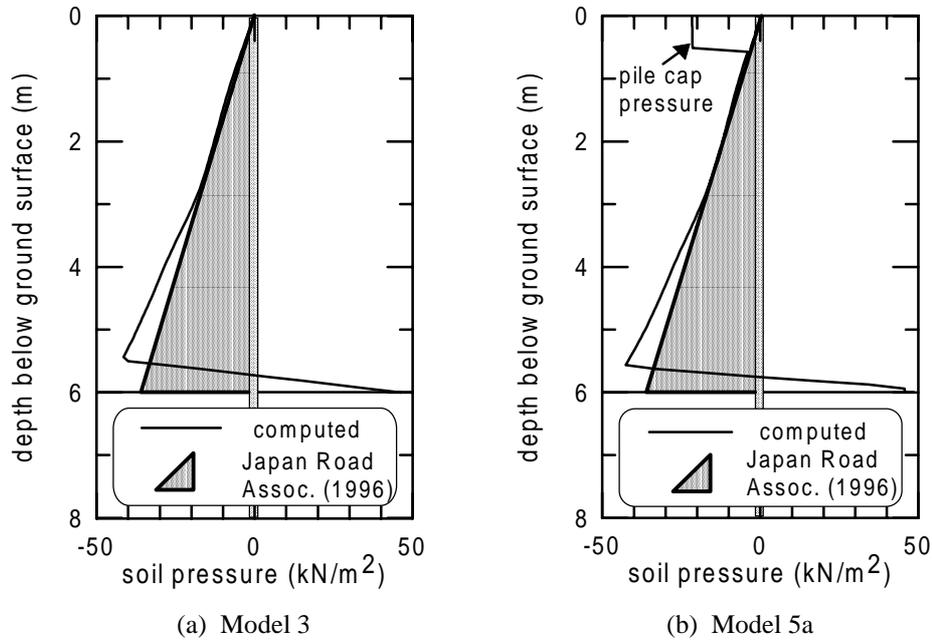
**Figure 9 Comparison of BSTRUCT Pressure Diagrams with Japan Road Association's Recommendations**
