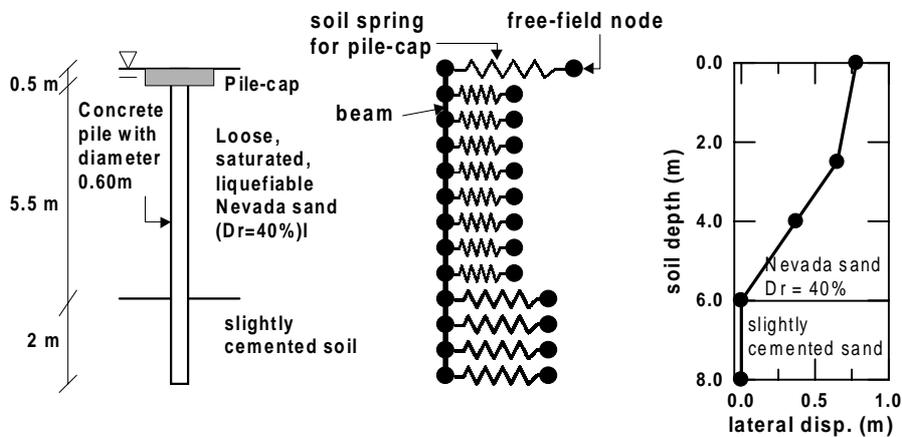
(a) Model 5a Soil-Pile-Cap System (b) Finite Element Model (c) Free-Field Lateral Displacements
