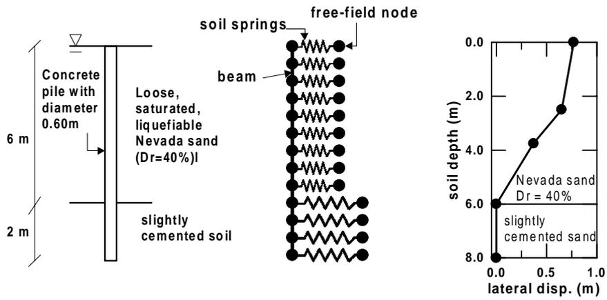
(a) Model 3 Soil-Pile System (b) Finite Element Model (c) Free-Field Lateral Displacements
