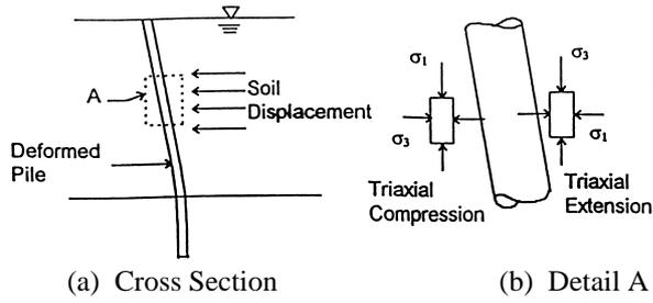
**Figure 1 Schematic of Relative Soil-Pile Movement and Analogous Triaxial Loading Conditions**
