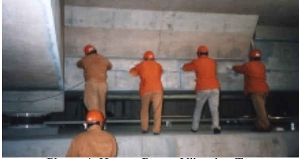
Photo. 4 Human Power Vibration Test
