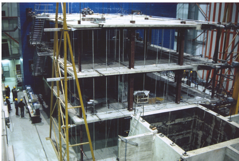
Figure 2: View of tested 3-D frame in front of reaction wall at ELSA facility
