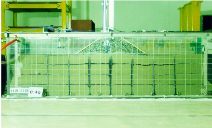
Photo 1. Deformed embankment of case 11 after 0.4g excitation
