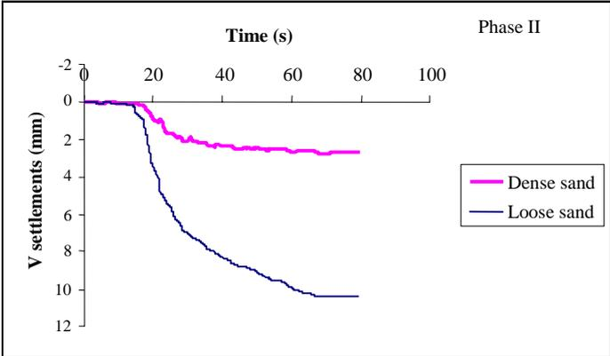
Fig. 5: Phase II: Vertical displacement of the foundation.
