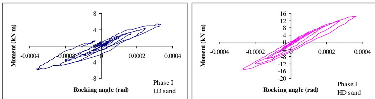
Fig. 3: Phase I: overturning moment vs. rocking for LD (left) and HD (right) soil conditions
