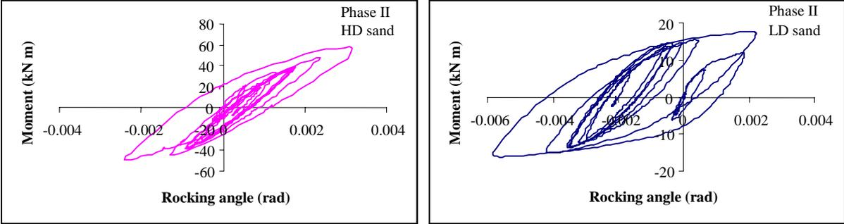
Fig. 4: Phase II: Overturning moment vs. rocking for HD and LD conditions.
