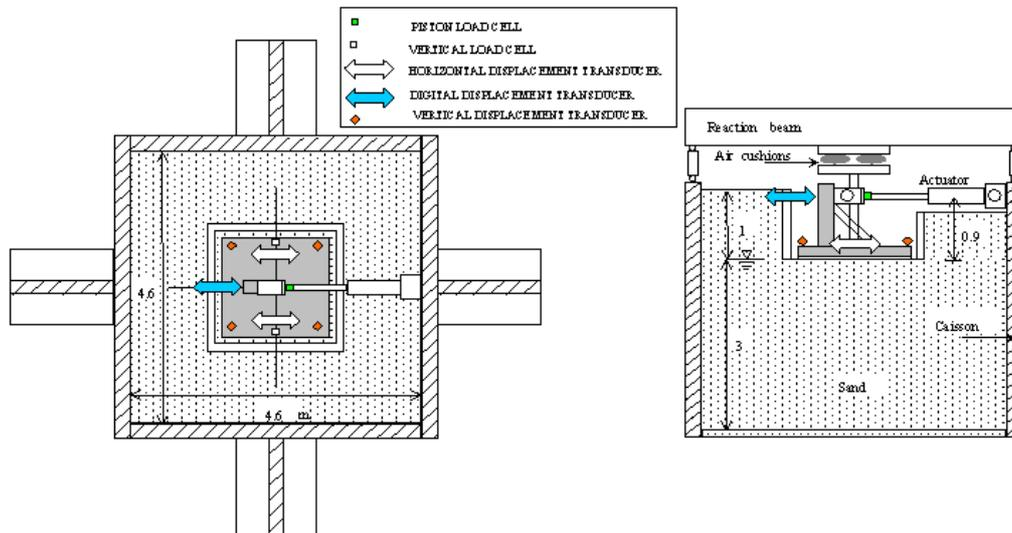
**Fig. 1: Scheme of the experimental setup.**
