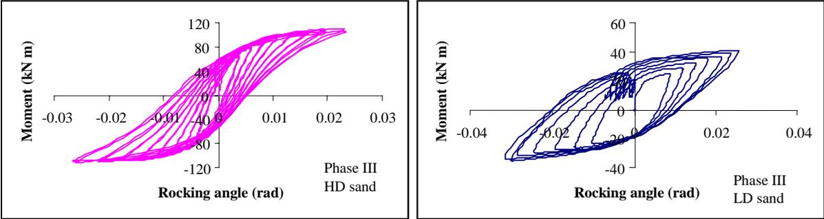
**Fig. 6: Phase III: Overturning moment vs. rocking for HD and LD conditions.**
