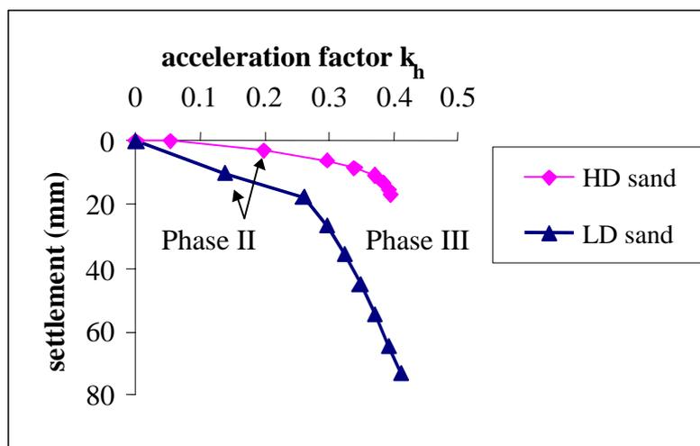
**Fig. 8 - Comparison of foundation settlements in HD and LD soil conditions as a function of the seismic coefficient ( $k_n=H_{max}/V$ ).**
