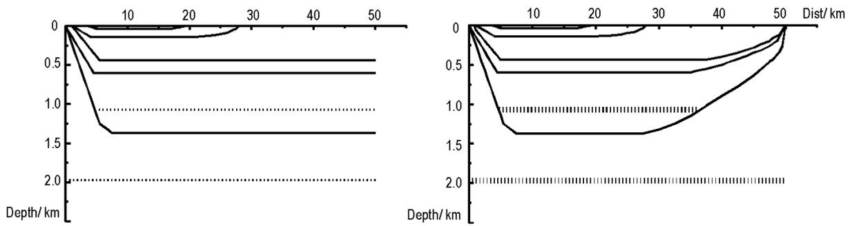
**Figure 5 – Layers geometry of the Lower Tagus Valley basin. (a) On the left: structural model estimated from the geological and the geotechnical characterisation; (b) on the right: simplified structural model used in the numerical computations. The maximum thickness of the shallower layer is 40 m. S-wave velocities for the different layers are: V1= 230 m/s; V2= 750 m/s; V3= 1150 m/s; V4= 1330 m/s; V5= 1550 m/s; V6= 1730 m/s; V7= 2900 m/s; V8= 3500 m/s (basement).**
