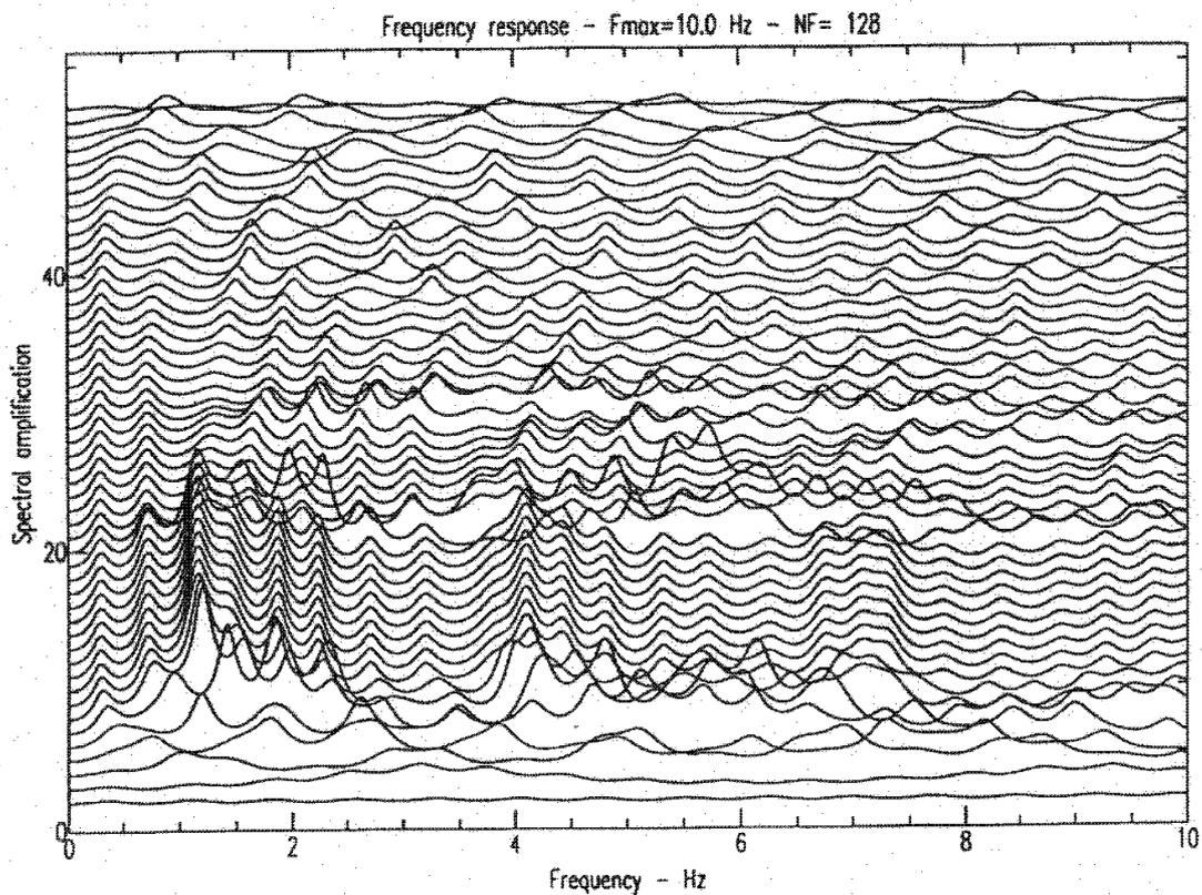
**Figure 6 – Spectral amplification obtained for 50 points equally spaced along the cross-section valley, using the Thomson-Haskell 1D modelling.**
