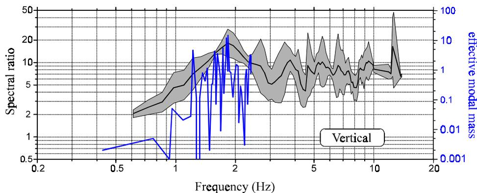
**Figure 8 Experimental vertical spectral ratio (left) and percentage of effective modal mass (right) vs frequency**
