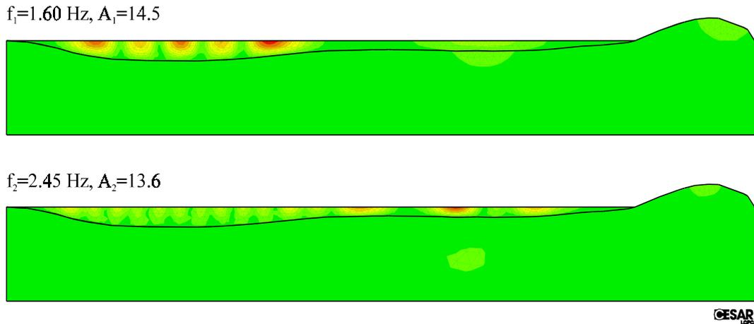
Figure 2. Estimation of amplification factor for a vertical SH-wave at different frequencies.
