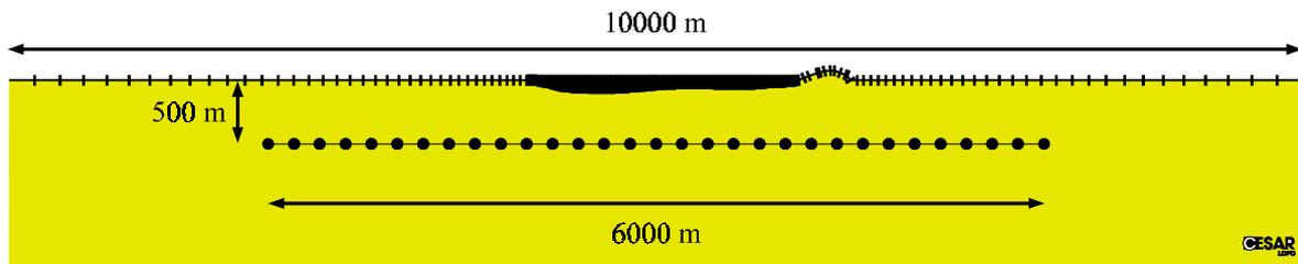
**Figure 4. Boundary element mesh for P and SV waves.**
