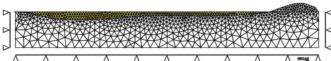
**Figure 5. Finite element mesh for the determination of eigen modes.**
