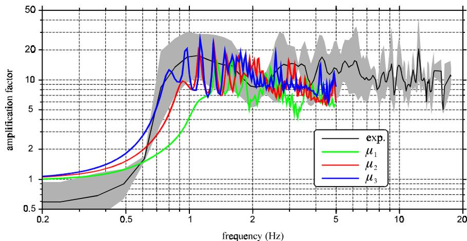
Figure 3. Maximum amplification factor vs frequency for three different shear moduli of the alluvial layer (comparison with experimental results).
