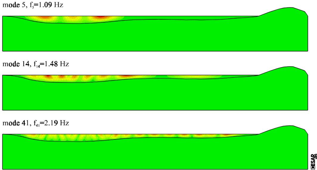
Figure 6. Eigenmodes and eigenfrequencies (5th, 14th and 41st) of the basin.
