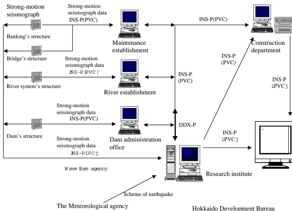
**Figure 3-3-1 Configuration of the network**
