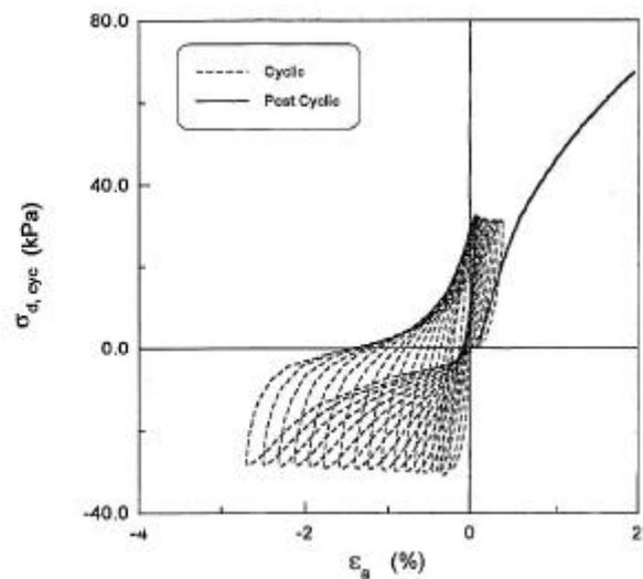
Figure . Cyclic and Post-Cyclic stress-strain Results for sample #6A
