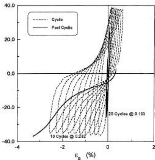
Figure 4. Cyclic and Post-Cyclic stress-strain Results for sample #6A
