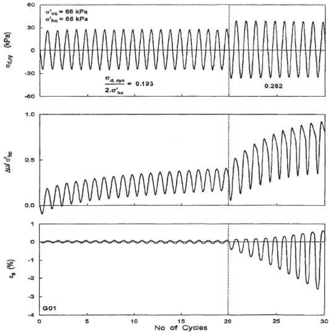
Figure 3. Results of Cyclic Testing of sample #6A
