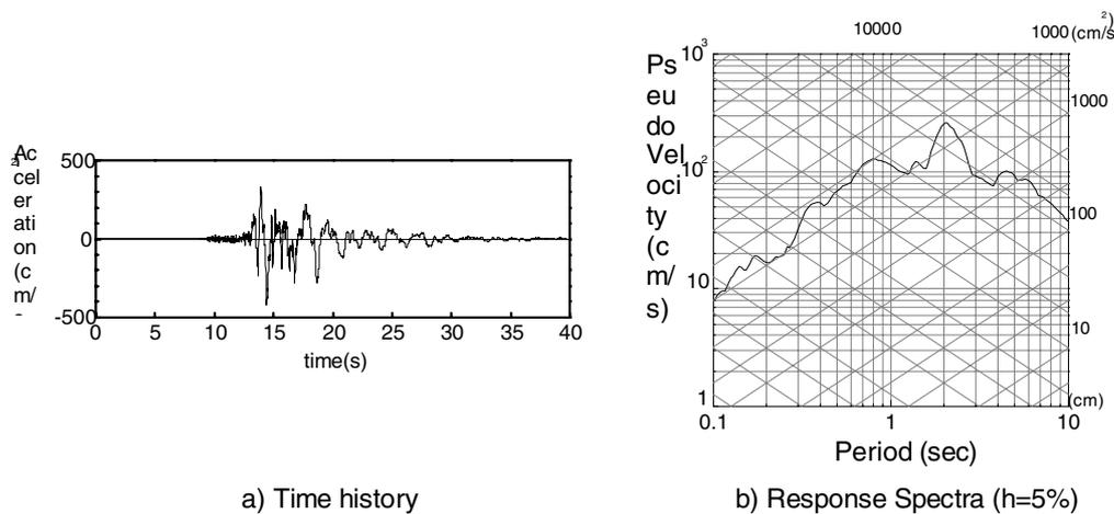
**Figure 6: Input motion of analysis (Observed record of GL-34m at EKB)**
