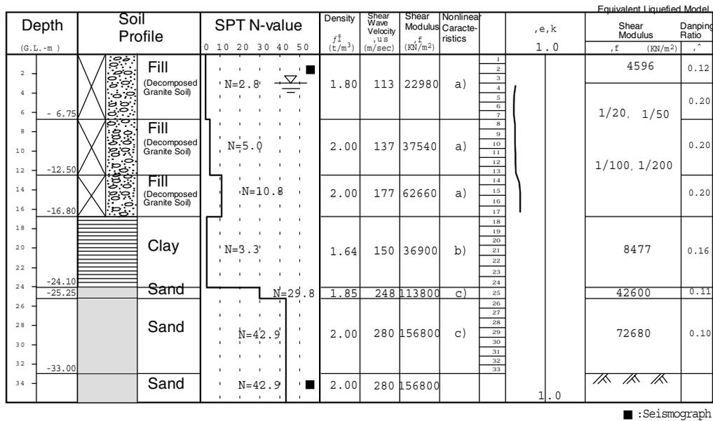
**Figure 2: Soil Profile at East Kobe Bridge**
