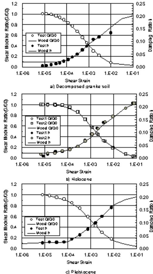
Figure 4: Relation of shear modulus and damping ratio versus shear strain
