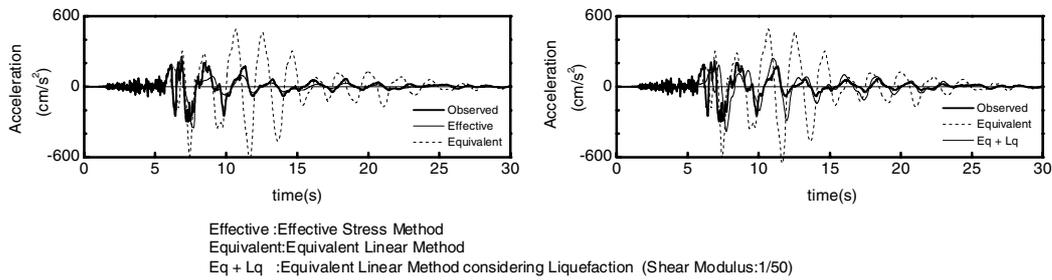
**Figure 7: Comparison of acceleration time histories at the surface (East Kobe Bridge)**
