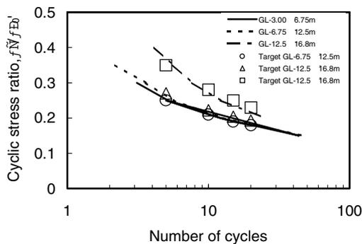
Figure 5: Liquefaction resistance of reclaimed fill (Masado)
