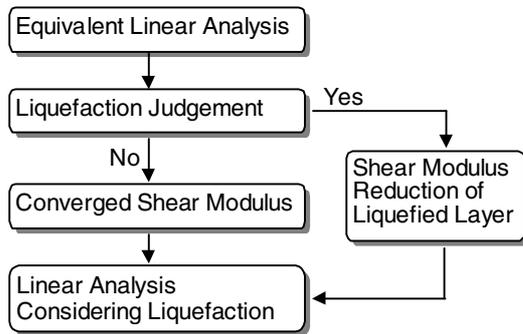
Figure 3: Procedure of equivalent linear analysis considering liquefaction
