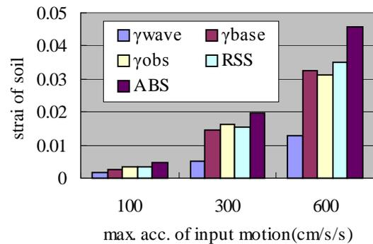
Figure 5: Maximum strain of soil observed by tests
