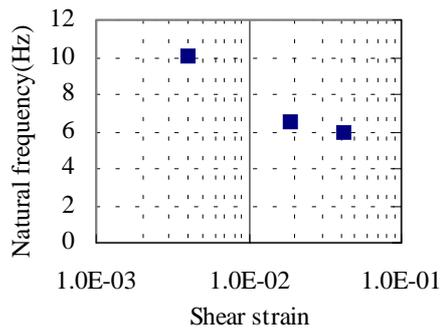
**Figure 3: Natural frequency versus shear strain of soil**
