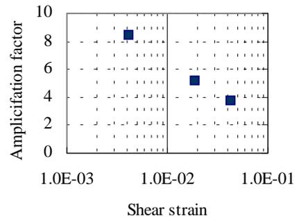
**Figure 4: Amplification factors versus shear strain of soil**
