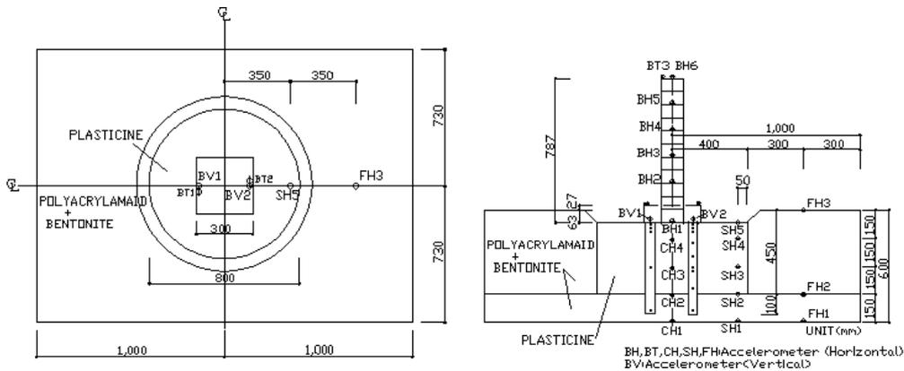
Figure 2: Test model and measurement apparatus
