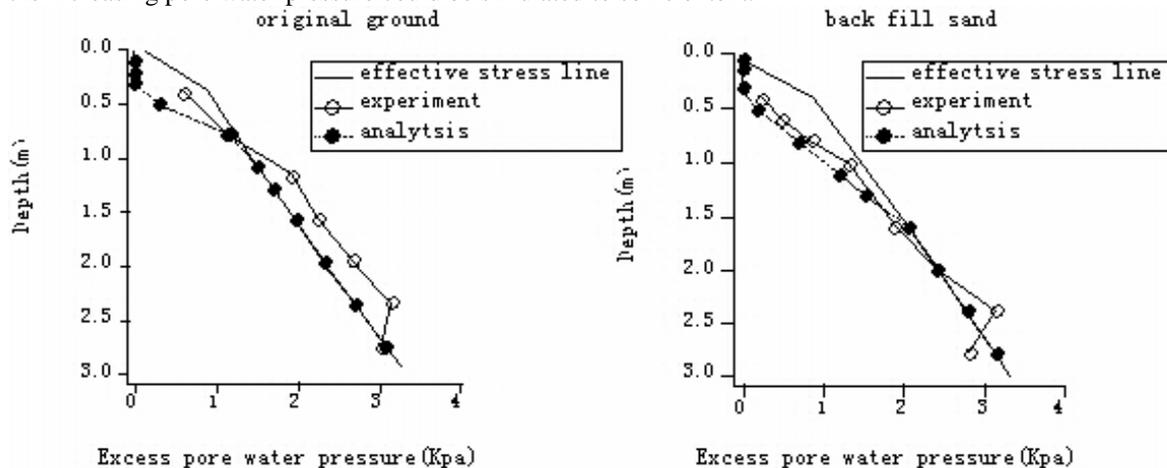
Figure 6 Maximum excess pore water pressure distribution in Exp.3
