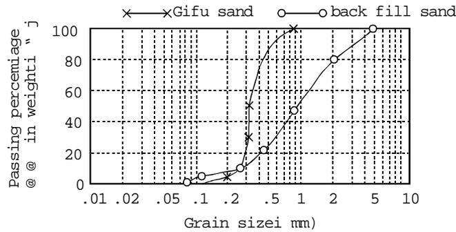
**Figure 2 Grading curves of sand**
