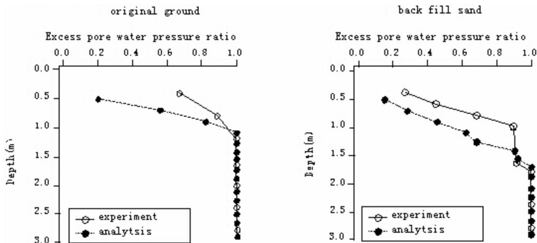
Figure 7 Maximum excess pore water pressure ratio in Exp.3
