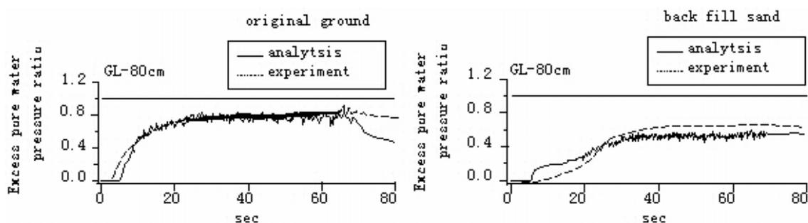
Figure 8 Time histories of excess pore water pressure ratio wave in Exp.3
