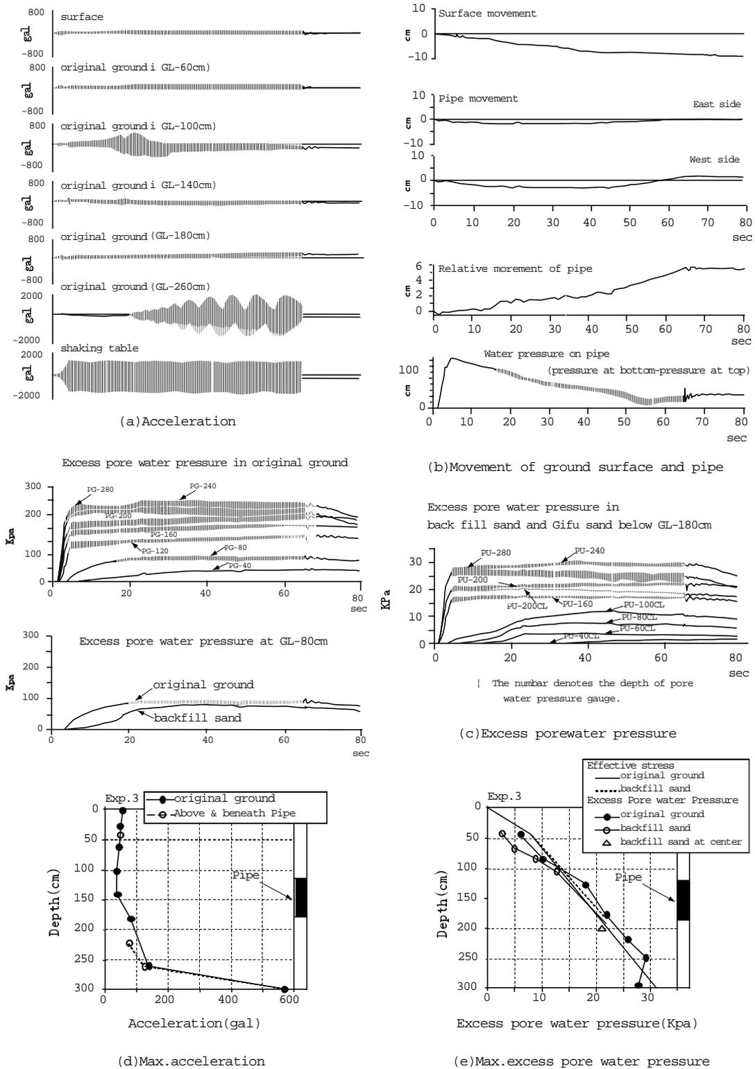
Figure 3 Time histories of acceleration, pipe movement, excess pore water pressure, etc. in Exp.3
