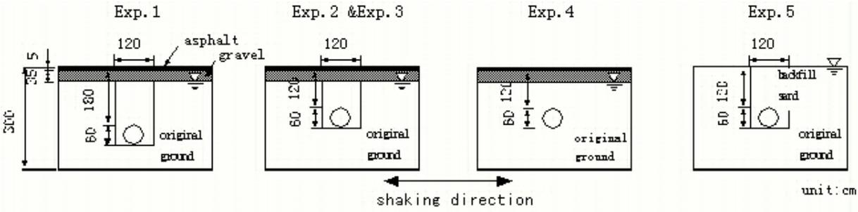
Figure 1 Key sketches of the vertical section in experiment
