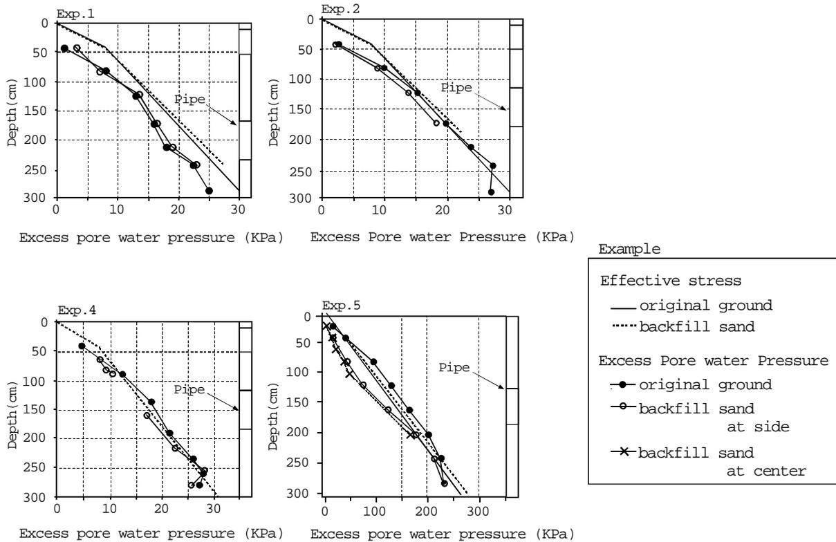
**Figure 4 Maximum excess pore water pressure distribution**
