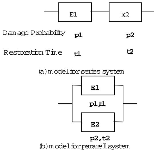
**Figure 1 Illustration of serial and parallel system**
