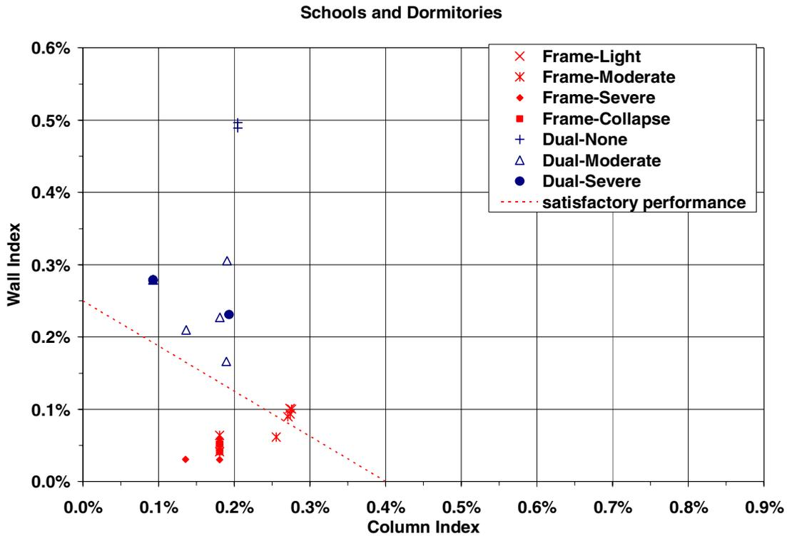
**Figure 16. Correlation between the structural performance and the wall and column indexes defined by Hassan and Sozen (1997).**
