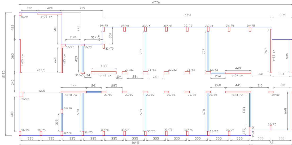
**Figure 13. Structural floor plan for building C-17-03. Masonry wall thickness was 0.19m. Dimensions are in cm.**
