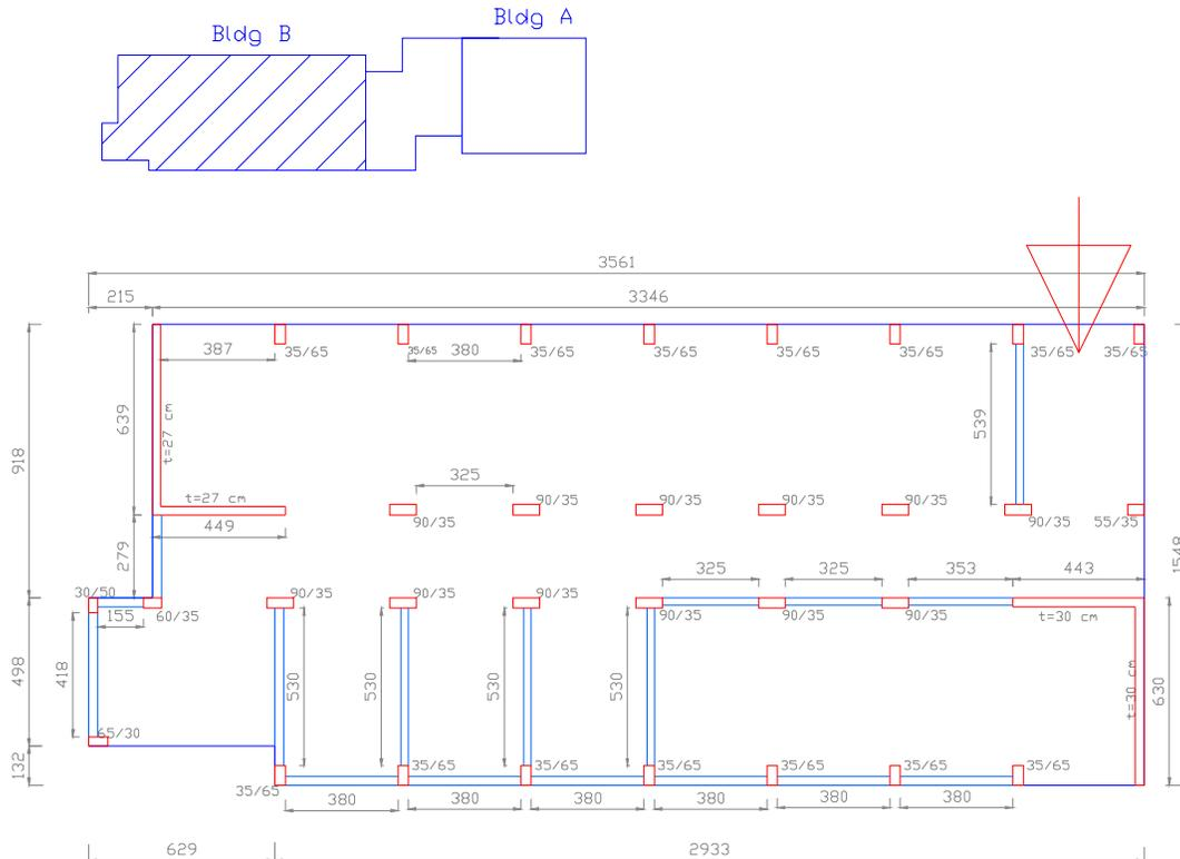
**Figure 11. Structural floor plan for building C-14-08. The thickness of interior and exterior masonry walls were 0.25m and 0.3 m, respectively. The arrow shows the entrance to the building. Dimensions are in cm.**
