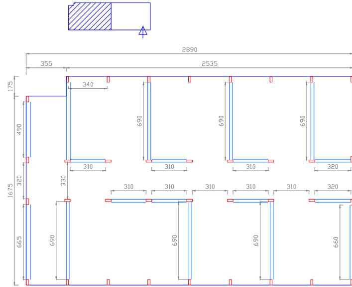
**Figure 6. The floor plan for C-12-02. The structural system is a moment-resisting frame. The columns are 0.2m x 0.5m. The school building comprises two independent structures separated by an insufficient expansion joint. Only the shaded part in the upper figure was surveyed. The arrow indicates the entrance to the building. The dimensions are in cm.**
