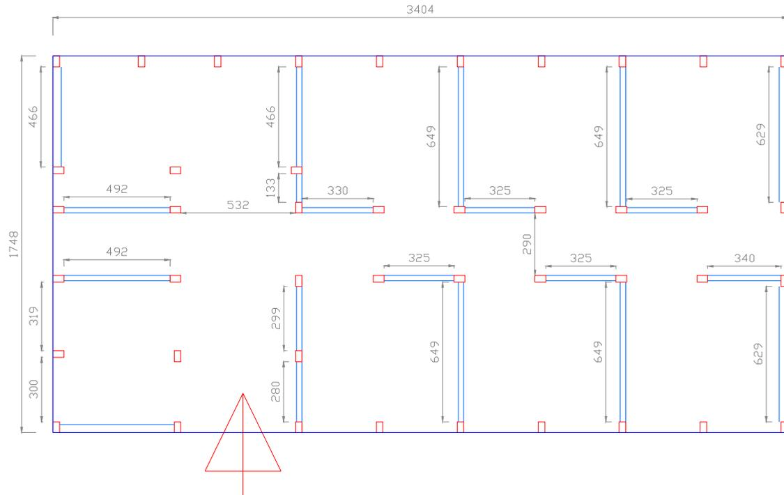
**Figure 4. Typical school plan without shear walls. All the walls shown in the drawing refer to those occupying a full span. Walls with openings are excluded. All the columns have dimensions of 0.3m x 0.5m. The arrow indicates the entrance to the building. Dimensions are in cm.**
