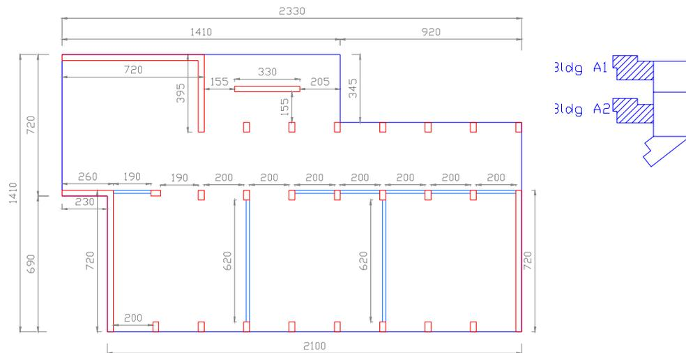
**Figure 10. Structural floor plan for building C-13-04A. All the columns have dimensions of 0.3m x 0.5m. The thickness of the reinforced concrete and masonry walls were 0.3m and 0.16m, respectively. Dimensions are in cm.**
