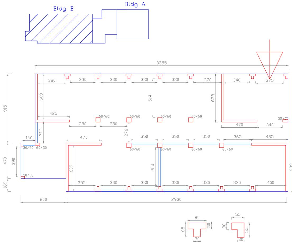
**Figure 12. Structural floor plan for building C13-03. The thickness of the shear walls was 0.3m. The masonry wall thickness was 0.25m for the interior walls and 0.3m for the exterior walls. The arrow shows the entrance to the building. Dimensions are in cm.**
