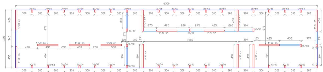
**Figure 14. Structural floor plan for dormitory buildings. The masonry wall thickness was 0.3m. Dimensions are in cm.**
