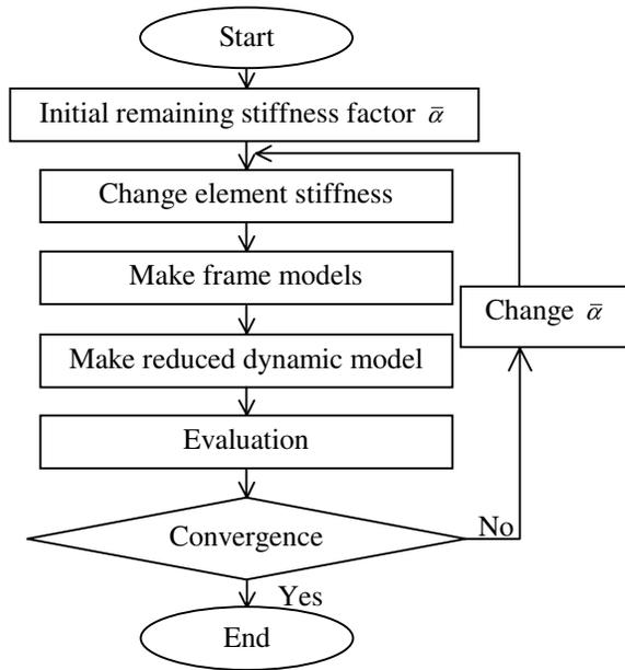
Fig.10 Flow chart of system identification
