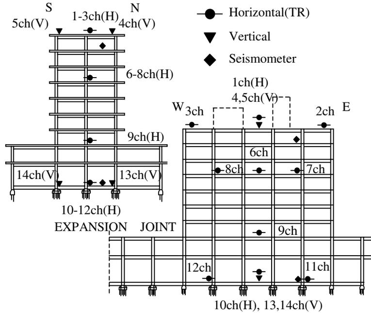
Fig.6 Sensor location for TR excitation
