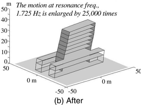
Fig.9 Comparison of fundamental modes of the two tests for LN excitation
