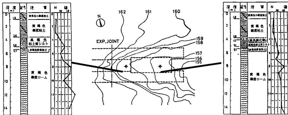
Fig.3 Original topography at the construction site and soil profiles
