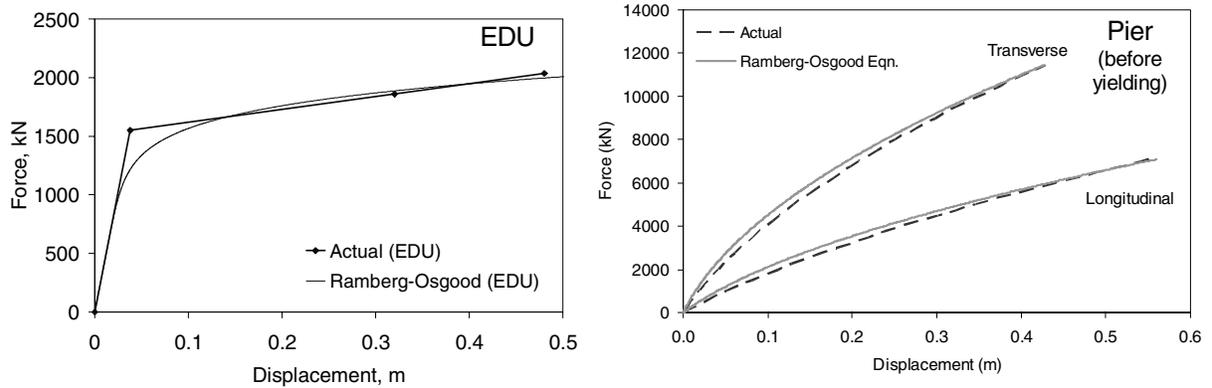
**Figure 10. The force-displacement characteristics of the members**
