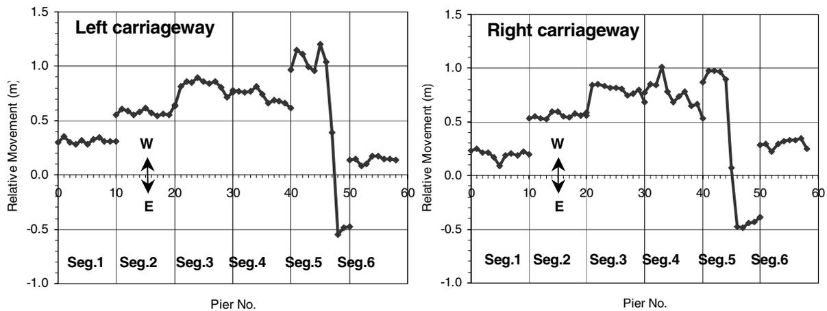
Figure 8. The relative movement of the girders with respect to the pier bases (ground)
