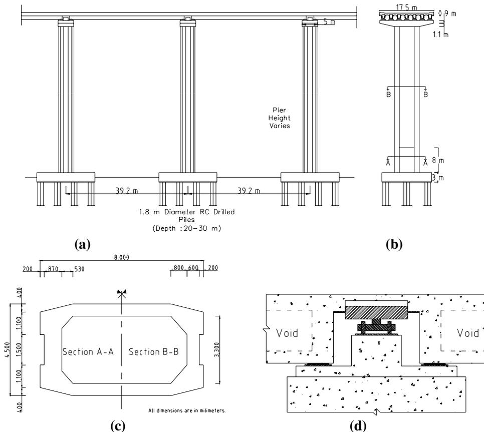
**Figure 3. Dimensions and details of the Bolu Viaduct. a) Side view, b) Transverse direction c) Pier cross sections, d) Side view of the joint between the deck and piers**
