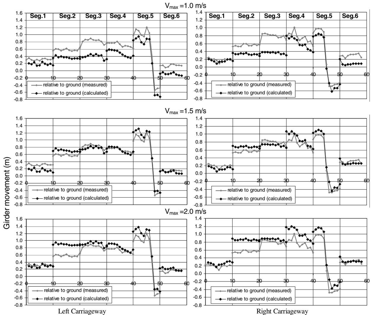
Fig. 16. Comparison of the results of analyses with the measurements of the deformed state of the structure.
