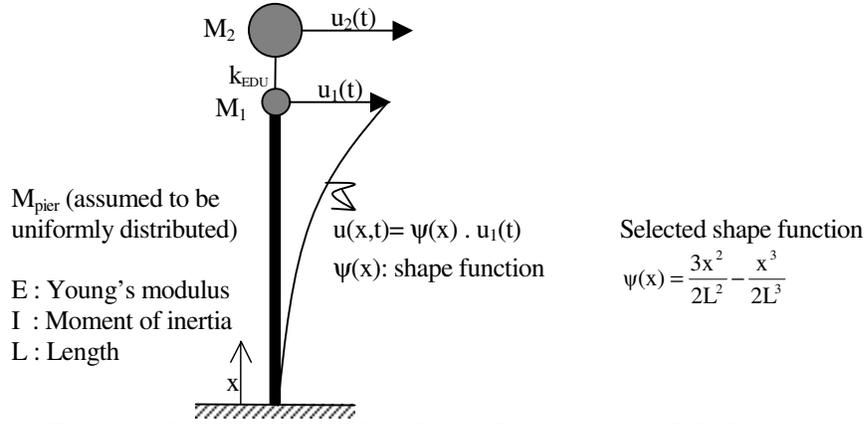
**Figure 9. Simplified model of the viaduct for ground shaking**
