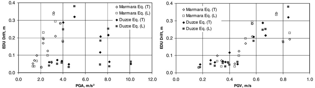
**Figure 12. The correlation of the maximum EDU drift with the PGA and PGV of the records**
