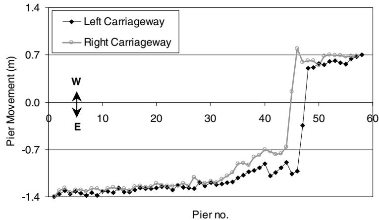
Figure 7. The measured movement of the piers in the longitudinal direction
