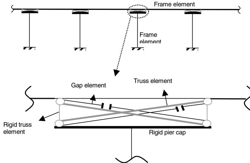
**Figure 13. The elements of the model of the viaduct for ground deformation analyses**
