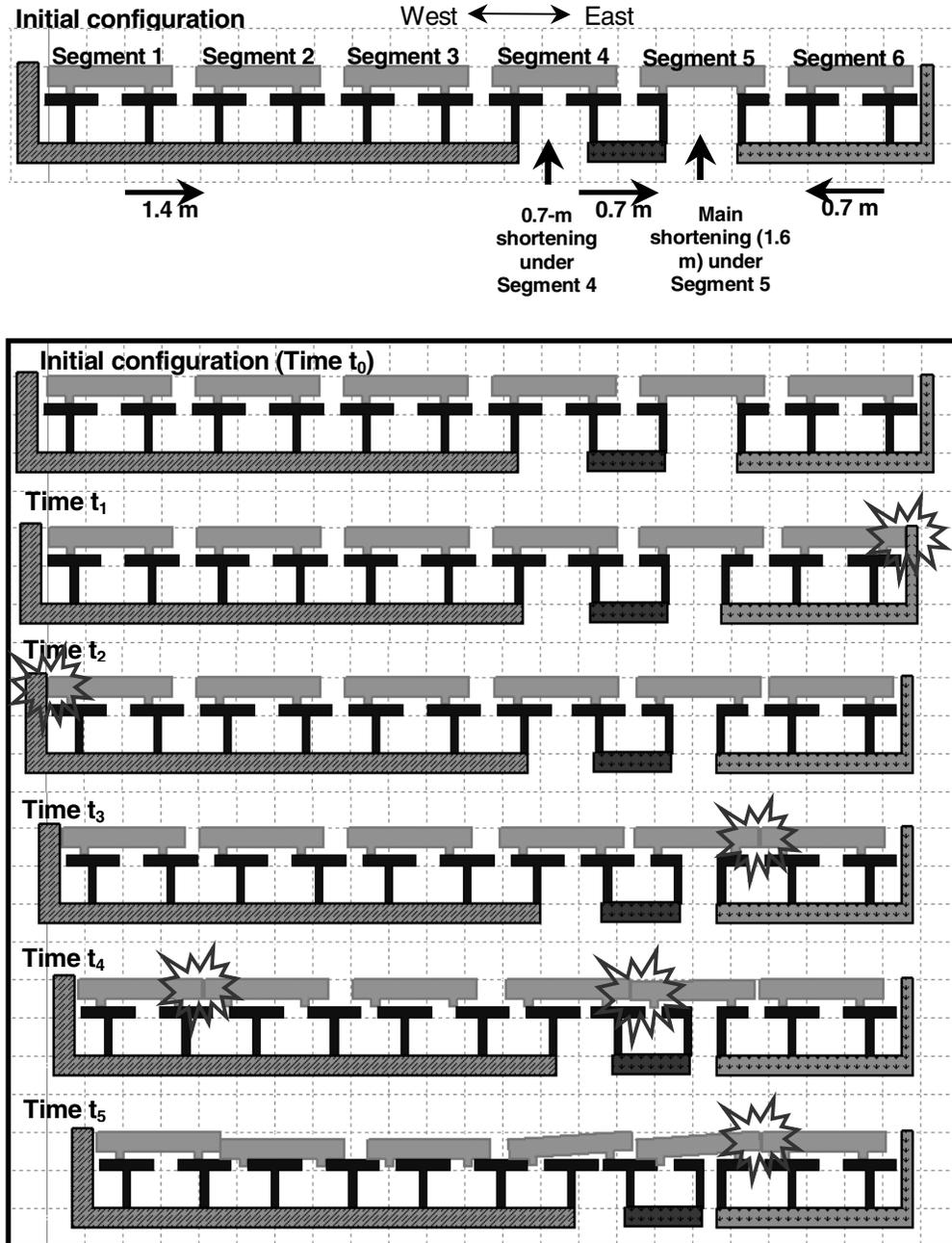
**Figure 15. Illustration of the dynamic response of the viaduct to the ground deformation. Each girder shown in the figure corresponds to one 10-span segment of the structure.**
