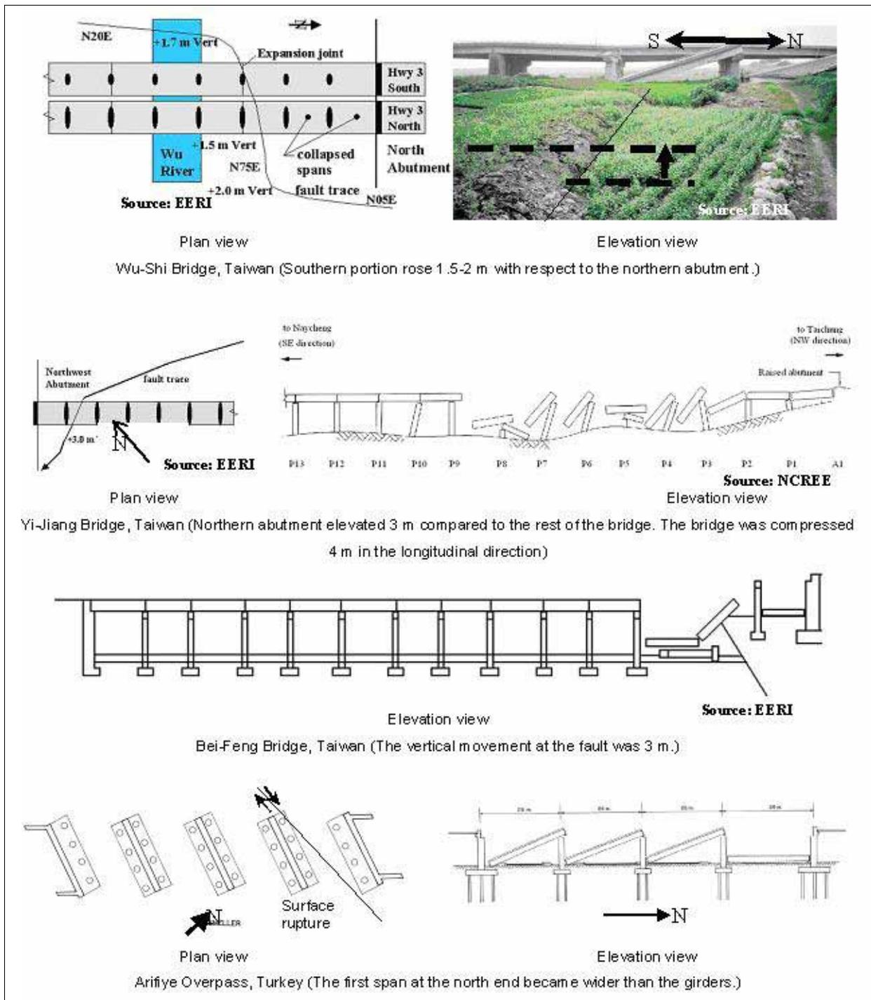
**Figure 1. The bridges in Taiwan and Turkey which collapsed during the 1999 earthquakes**
