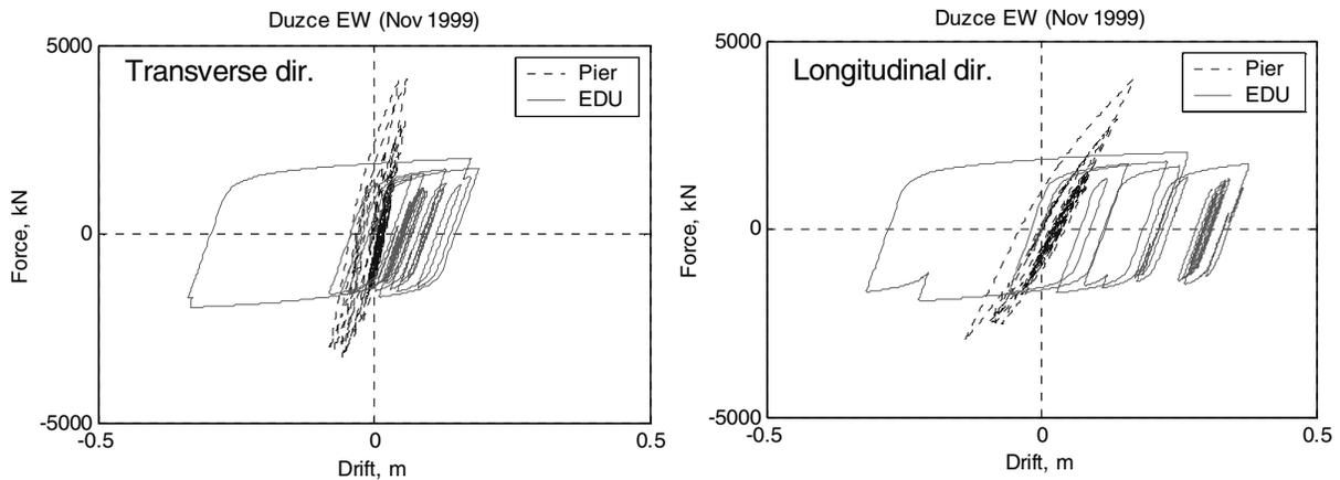
**Figure 11. The hysteresis curves of the elements in the analysis with record DZC-EW (Nov.)**
