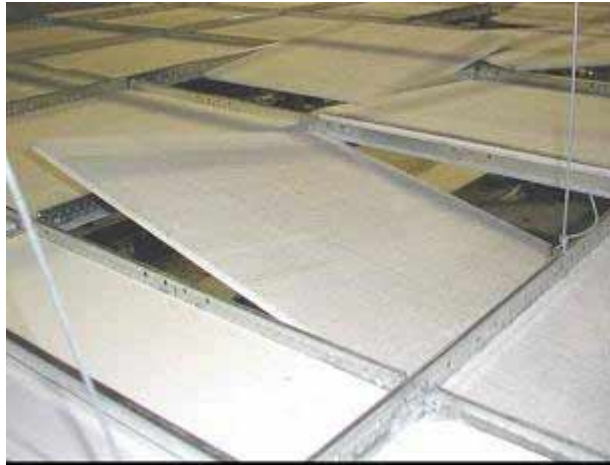
Figure 5. Tile rotating before falling, configuration 1
