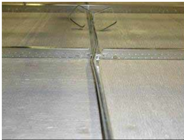
Figure 6. Buckling in 4-ft cross tees, configuration 2
