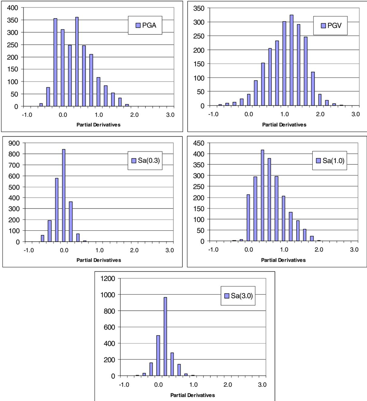
**Figure 7. Histograms of the partial derivatives of the scaled output with respect to the scaled inputs for the 3-story structure model. The model has a fundamental period of 0.6 sec.**
