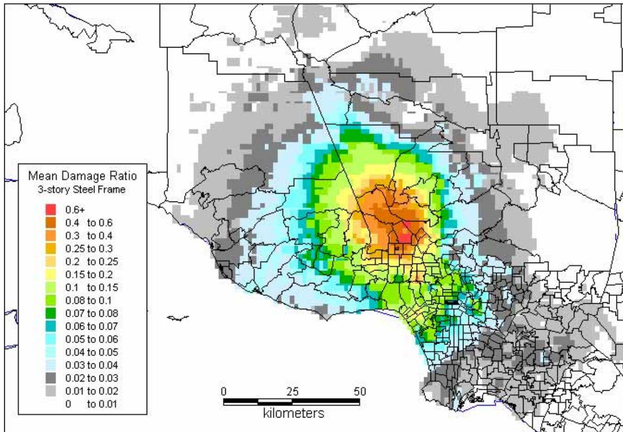
**Figure 8. Neural network prediction of MDRs for 3-story structure due to the Northridge earthquake**
