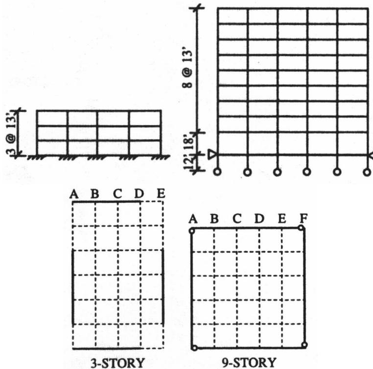
**Figure 1. Schematic figure of steel frame structure models used in this study (Gupta and Krawinkler [3])**
