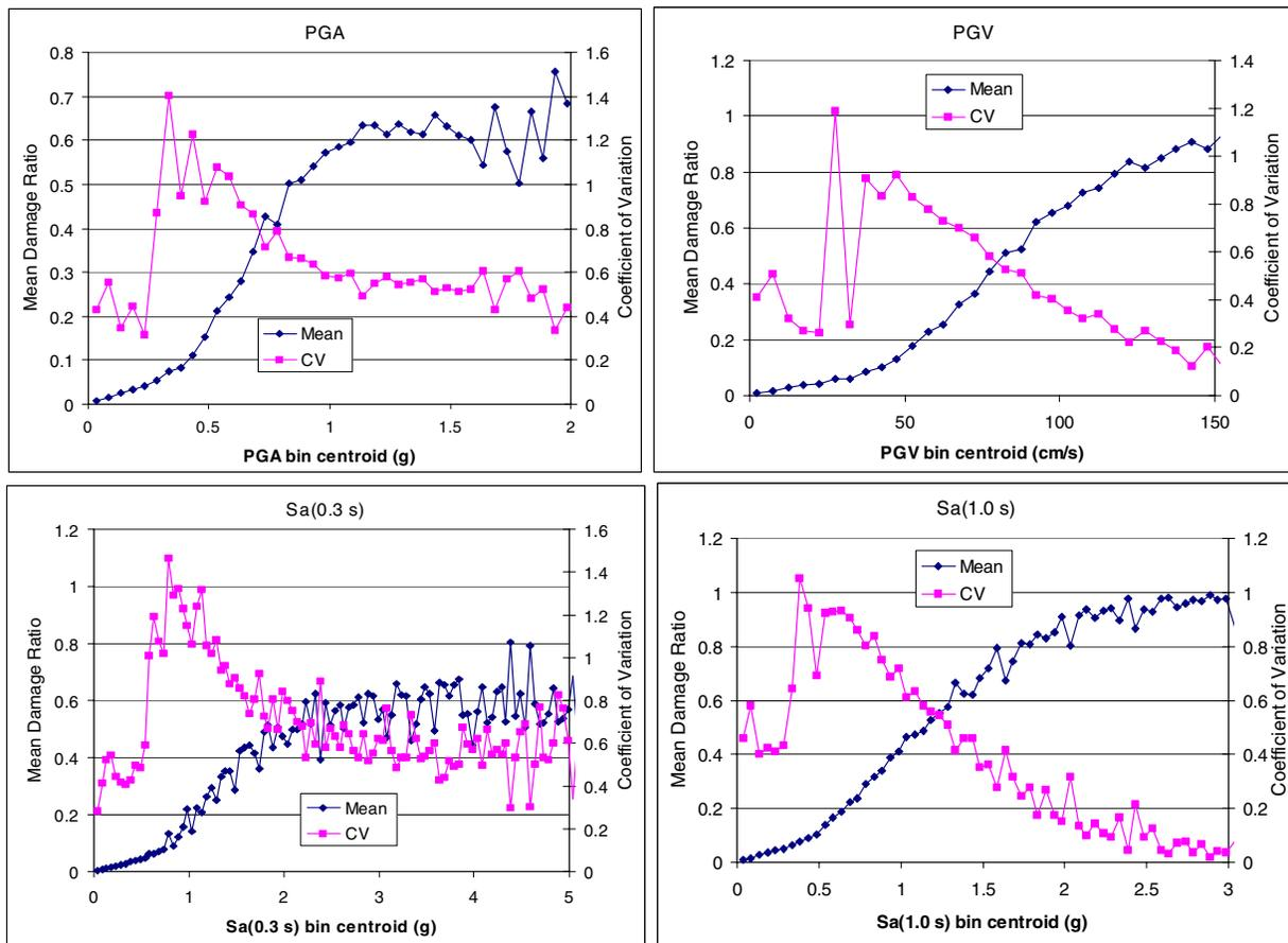
**Figure 3. Mean and coefficient of variation (CV) of the mean damage ratio per bin of the ground motion indices for the 3-story steel structure [clockwise from top left: PGA, PGV, Sa(1.0s), Sa(0.3s)]**
