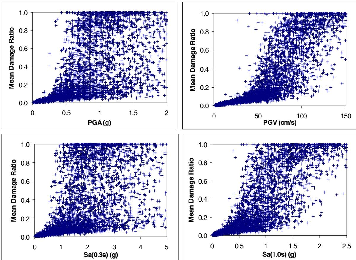
Figure 2. Distribution of calculated mean damage ratio of 3-story steel frame building model with respect to selected ground motion indices
