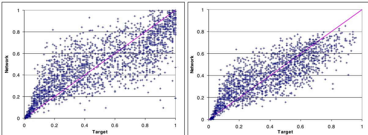
**Figure 6. Comparison of the target mean damage ratios with the network predicted mean damage ratios for the 3-story steel structure model (left) and the 9-story steel structure model (right.) This figure shows the data points for the training data only.**
