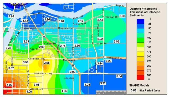
Figure 8. Thickness of Holocene sediments in the Fraser River delta (Richmond) overlaid with site periods obtained from SHAKE analyses
