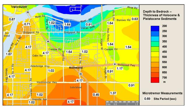
Figure 6. Combined thickness of Holocene and Pleistocene sediments in the Fraser River delta (Richmond) overlaid with site periods obtained from microtremor measurements
