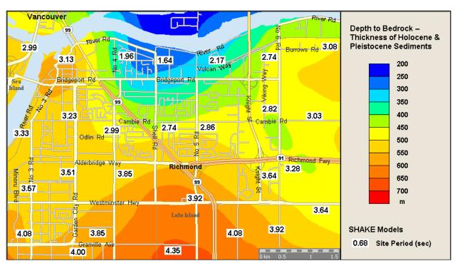
Figure 9. Combined thickness of Holocene and Pleistocene sediments in the Fraser River delta (Richmond) overlaid with site periods obtained from SHAKE analyses
