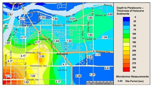
Figure 5. Thickness of Holocene sediments in the Fraser River delta (Richmond) overlaid with site periods obtained from microtremor measurements
