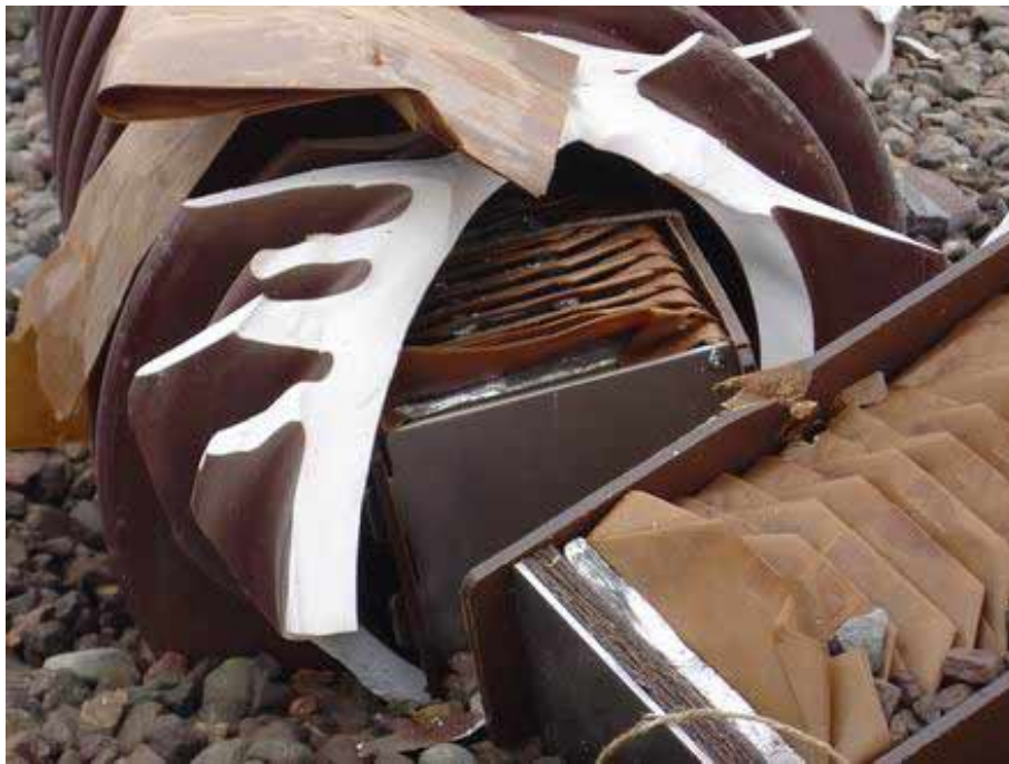
(Fig-4)- Porcelain part fall down and electrical internal components damaged
