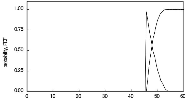
**Fig. 6. PDF and CDF of failure for Nojima Earthquake Fault**
