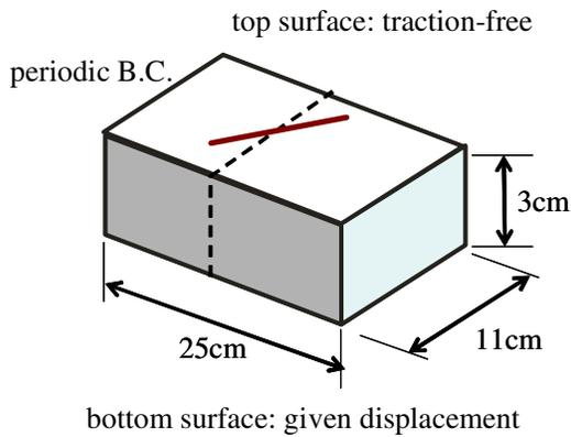
Fig. 1. SSFEM model for model
