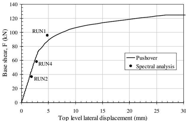
**Figure 6 Static pushover analysis force-displacement relationship**
