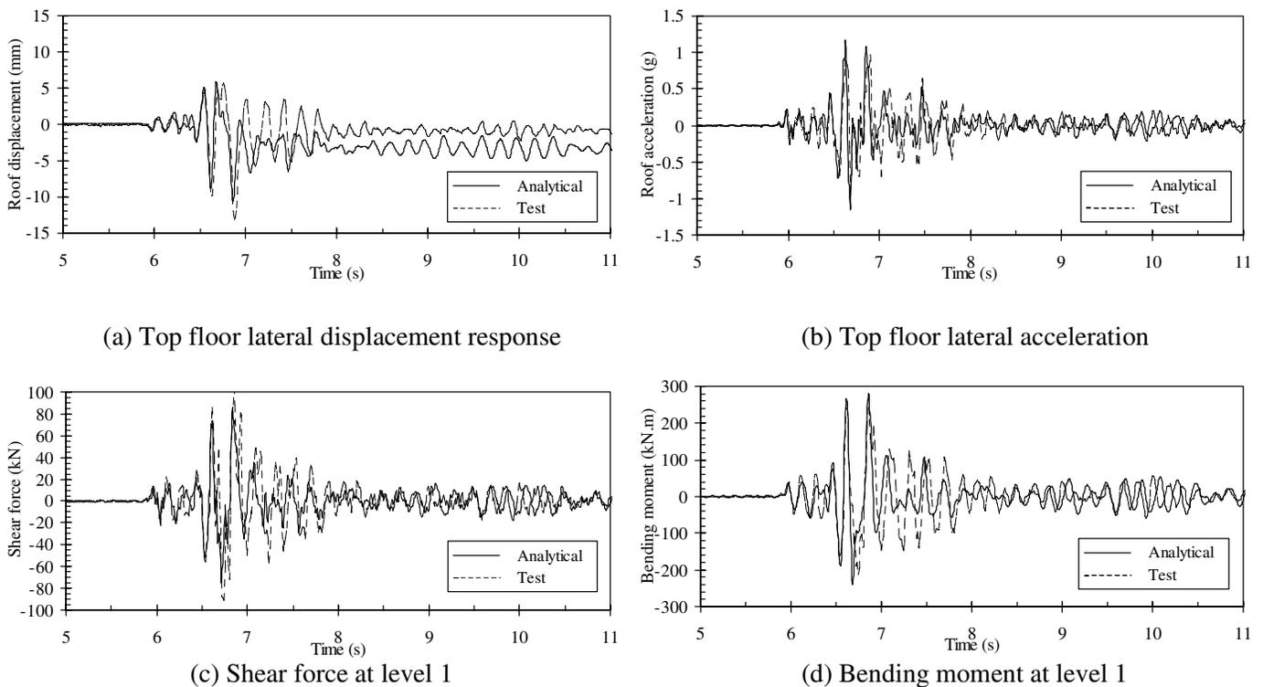
**Figure 13 Comparison between the predicted and measured responses for the test RUN3**
