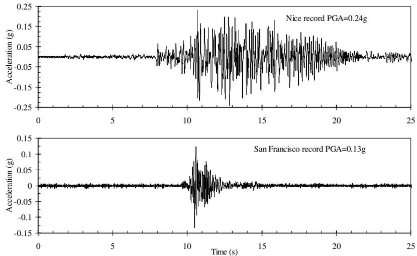
Figure 2 Measured accelerations on top of the shake table for the analysed runs
