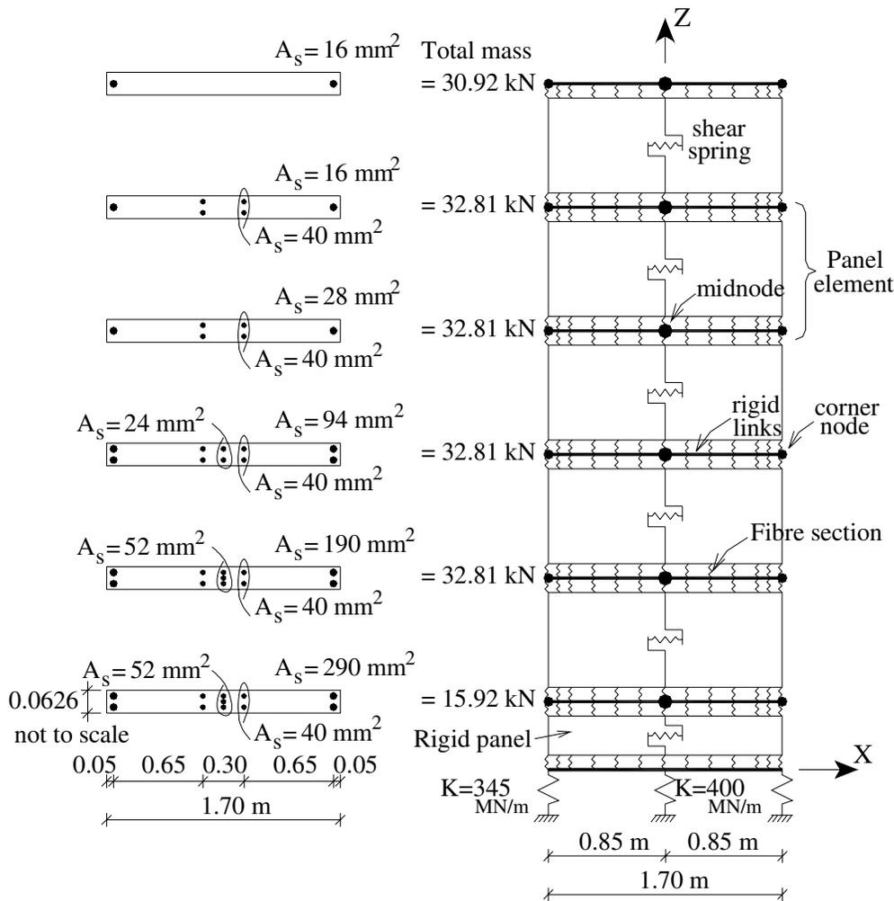
**Figure 12 Properties of the modeled tested wall**
