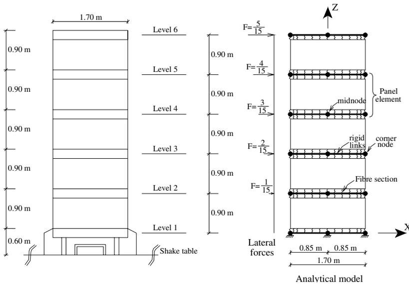
**Figure 4** Idealization of the tested wall for the pushover analysis
