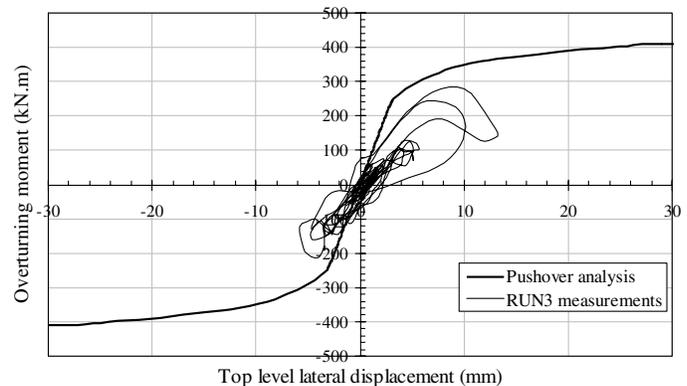
**Figure 7 Comparison between the pushover and RUN3 (the measured) moment-displacement relationships**
