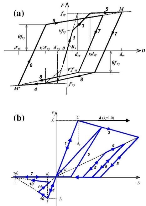
**Figure 5** (a) Hysteresis model for steel, SS3; and (b) Concrete material bilinear model, CS2. [2]
