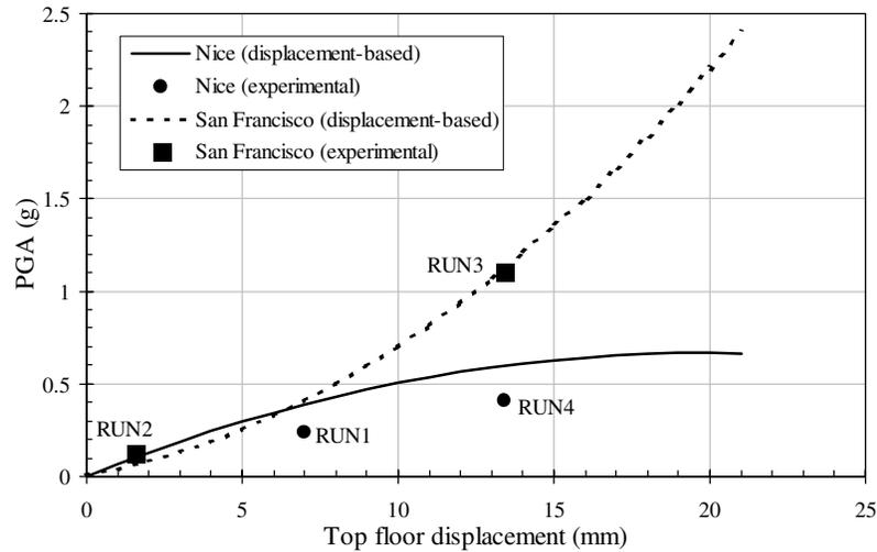
**Figure 11 Estimated PGA at target top floor displacements from the displacement-based approach versus results of the four tests**
