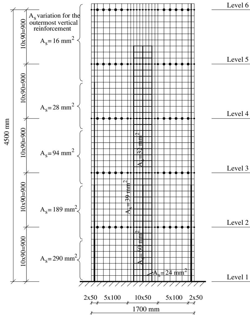
**Figure 8 Finite element model for spectral analysis**
