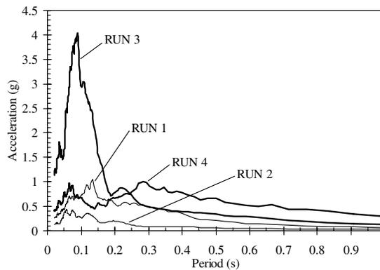
Figure 3 Response spectra for the four experimental runs.
