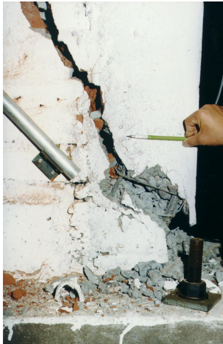
Figure 8. Final cracking for wall 4.
