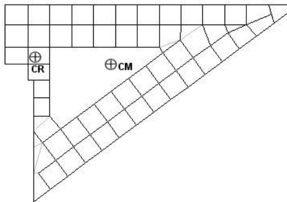
Figure 13. Plan view of the Building A showing the center-of-mass (CM) and center-of-rigidity (CR).
