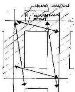
Figure 6. Masonry strut pattern for an infill masonry frame.
