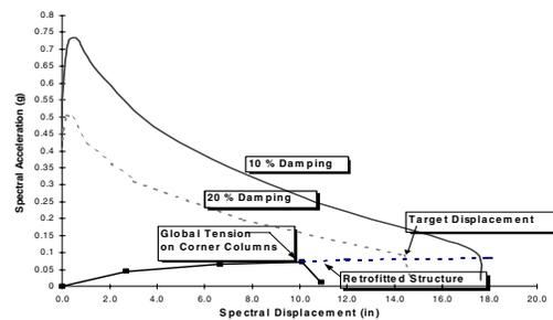
Figure 15. Demand and Capacity Spectrum for Building B – Y direction
