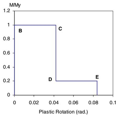
Figure 8. Beam-column connection backbone curve (FEMA 356).
