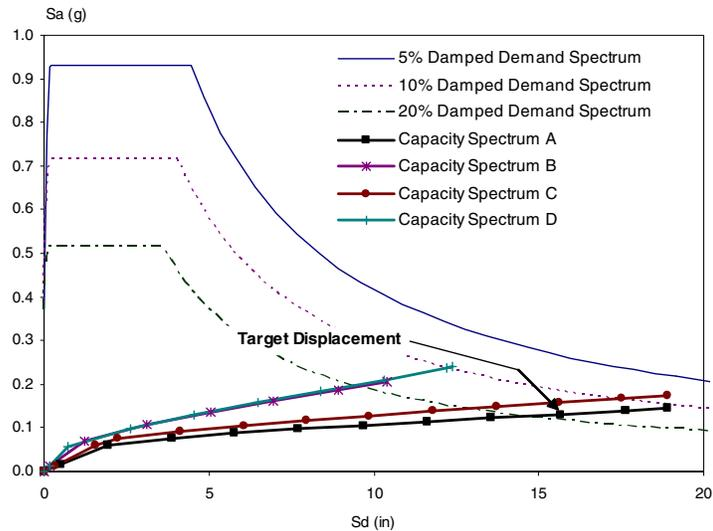
Figure 12. Demand and capacity spectra for Building A
