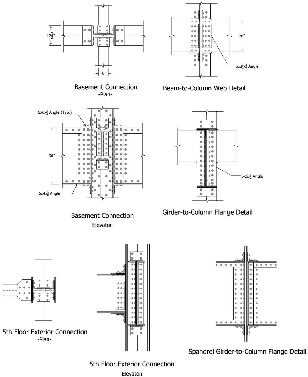
Figure 3. Building A Typical Connection Details.
