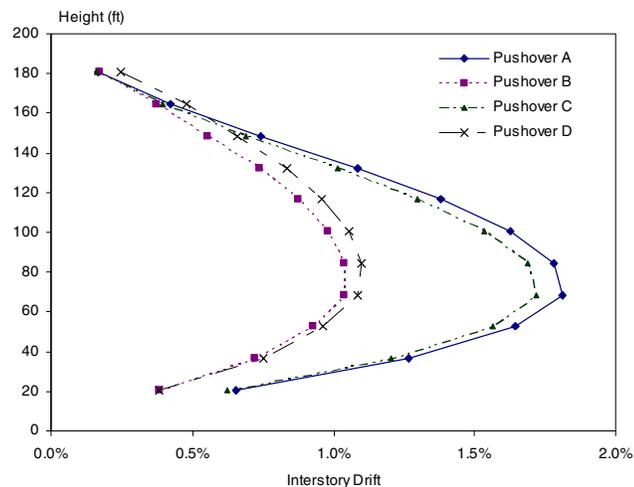
Figure 11. Inter-story drift ratios at the target displacement (orientations A and C) and instability point (orientations B and D).
