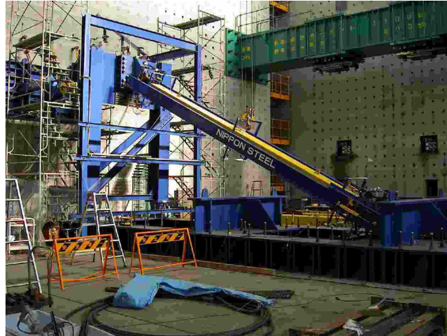
Figure 3.1 Photo of Test Setup for B-2 Brace
