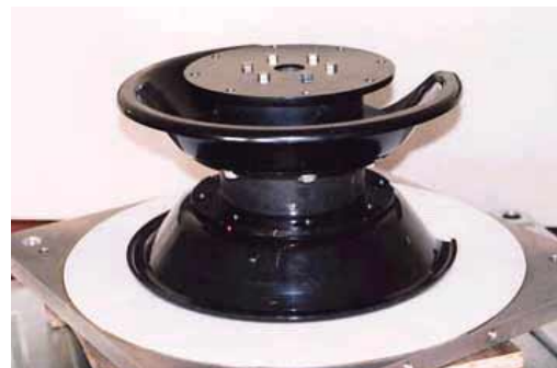
Photo 1 Isolator with buckling protecting plate
