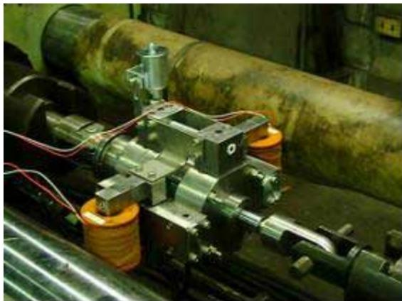
**Fig. 8 Double by-pass MR damper**
