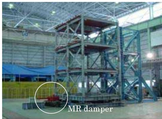
**Fig. 5 Three-story base-isolated structural model**
