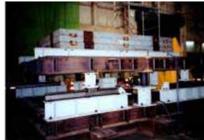
Fig.3 Picture of the Rigid base-isolated structural model
