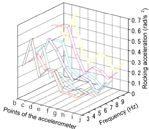
Fig.5 Relationship between excitation frequency and rocking acceleration (vertical and horizontal acceleration :200gal,
