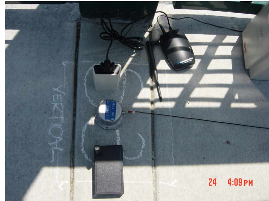
Figure 6. Going from top to bottom: ADXL 202E, traditional PCB 393C and, SD1221 sensor.
