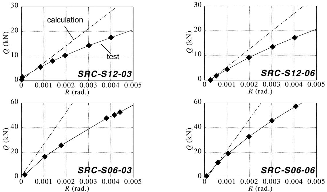
Fig.8 Comparison of Initial Rigidity
