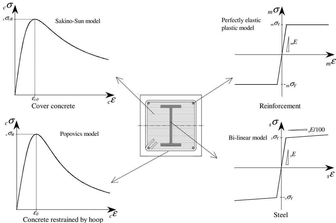
Fig.11 The Model of the Stress-Strain Relations
