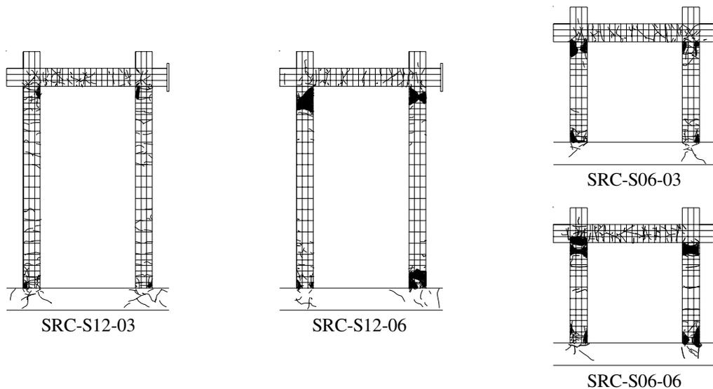
Fig.10 Crack Pattern (Final stage)
