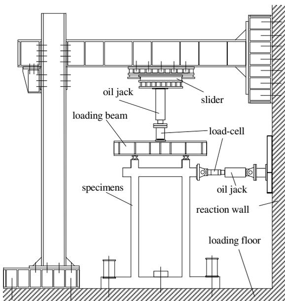
Fig.4 Loading Apparatus
