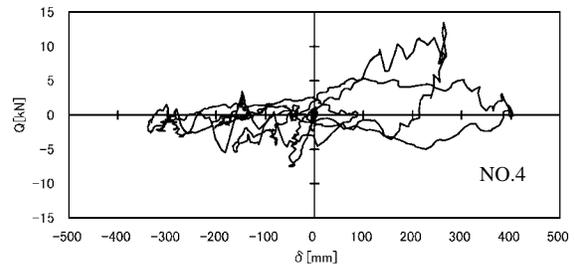
**Fig.4 the relationship between the load and deformation**
