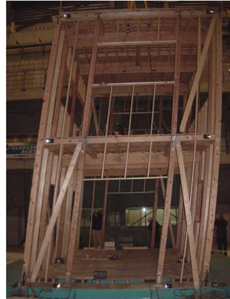
**Photo.2 Residual Displacement(No.4)**
