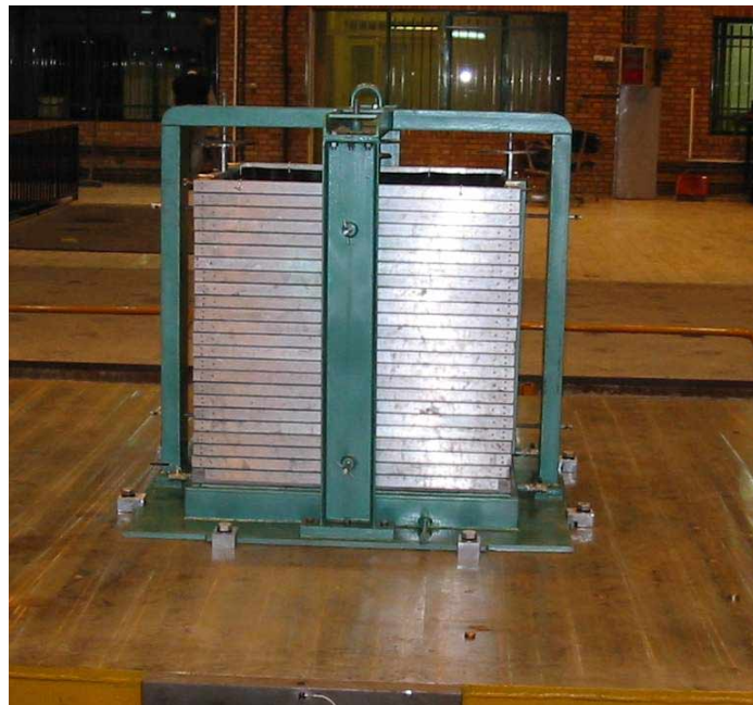
Figure 4: General view of the laminar shear box fastened on the shaking table
