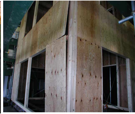
Fig.9 Separation of plywood-walls in first story.
