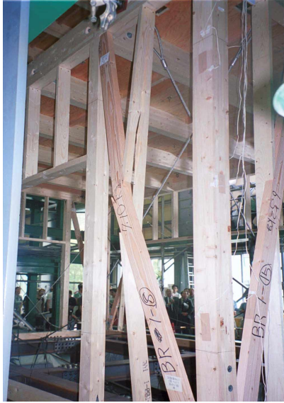
Fig.5 Break of wooden brace in first story.
