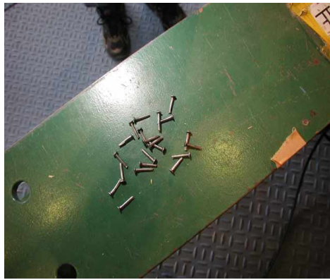
Fig.8 Fracture of nails used for plywood-walls.
