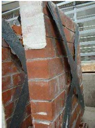
**Figure 5 Photo of specimen CDF1 showing the fabric debonded after failure**
